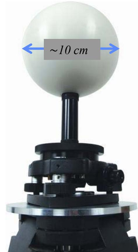
*Example of targets used in the registration of terrestrial laser scans (photos courtesy of leica-geosystems)*
