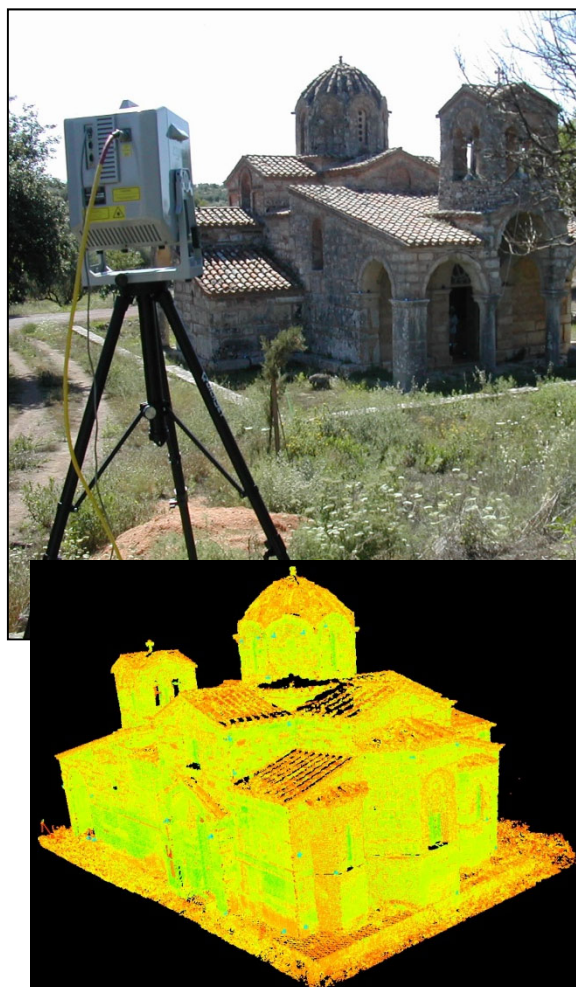
Static Terrestrial Laser Scanning
