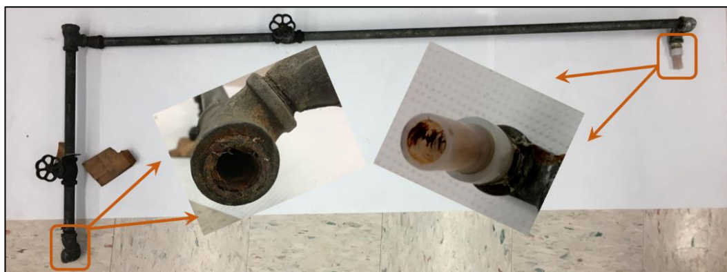
Figure 3.2 Image of metal scales on exhumed galvanized and PEX drinking water pipes from the cold city water supply line.
