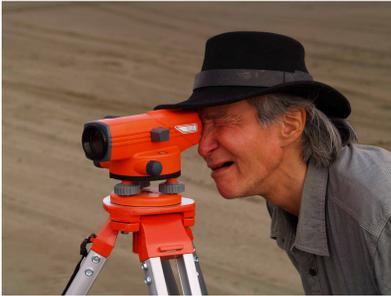
*An automatic level provides the data needed to measure the changes in beach slope.*
