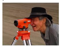
An automatic level provides the data needed to measure the changes in beach slope.
