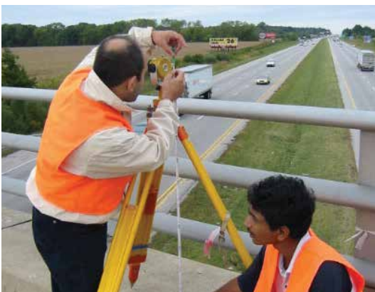
Geomatics graduate students conduct a control survey in preparation for static laser scanning. Photos courtesy of the School of Civil Engineering.
