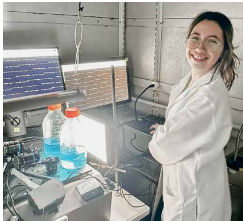
Amanda Lopez-Savage uses an automated IoT-enabled platform that integrates real-time intracellular lipid sensing and machine learning to monitor microalgal bioprocesses in the laboratory.
