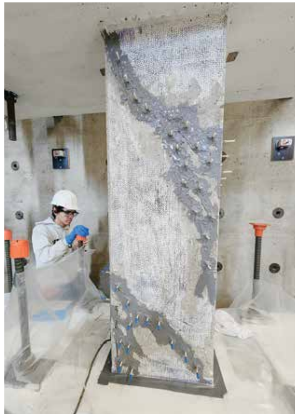
Lyles School of Civil and Construction Engineering graduate students test and review the seismic performance of concrete columns at the Robert L. and Terry L. Bowen Laboratory for Large-Scale Civil Engineering Research.
