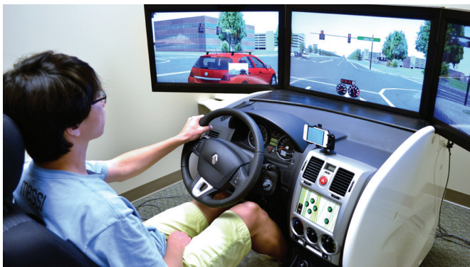
Graduate student Dong Yoon Song operates the Purdue Driving Simulator, which replicates automobile, traffic and weather conditions in and around Indianapolis. The DSL is located in the Purdue Technology Center. [Photo provided]
