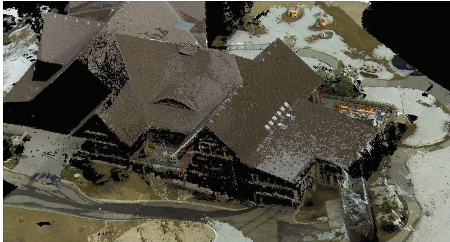
A sample point cloud over a building that has been derived from imagery collected via UAV.
