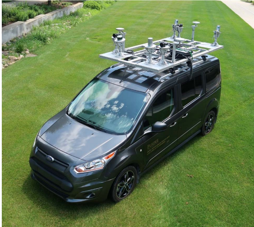
Purdue Wheel-based Mobile Mapping System (PMMMS)
