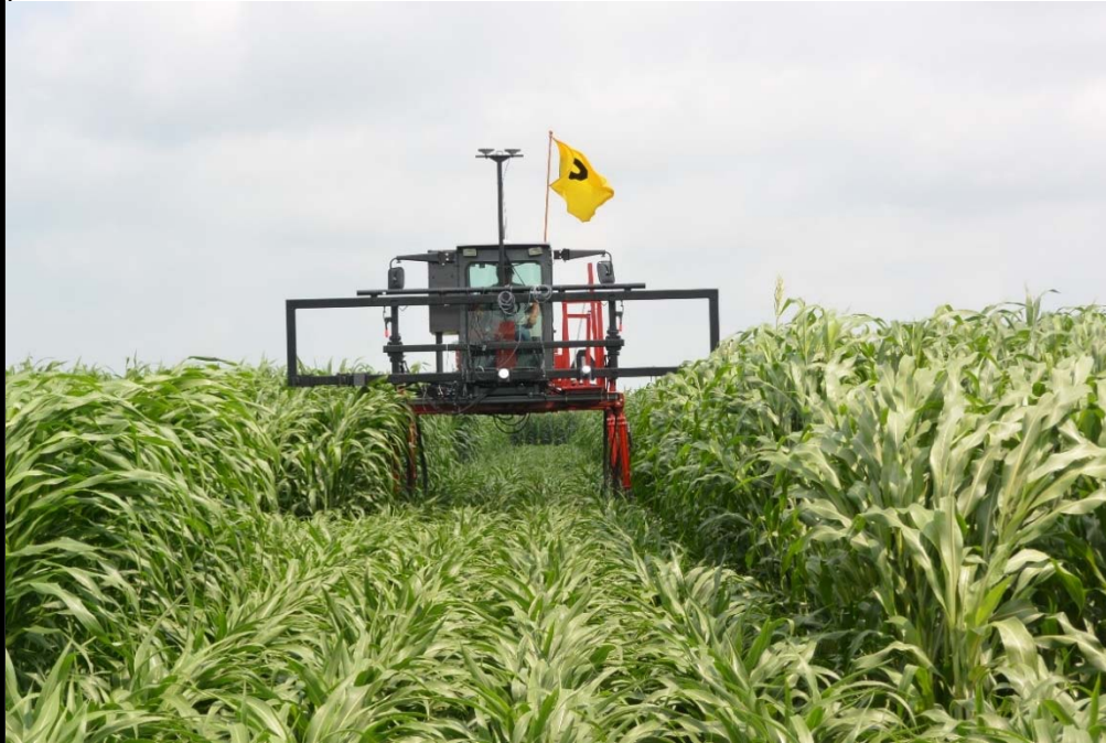
PhenRover: RGB, Hyperspectral, and LiDAR
