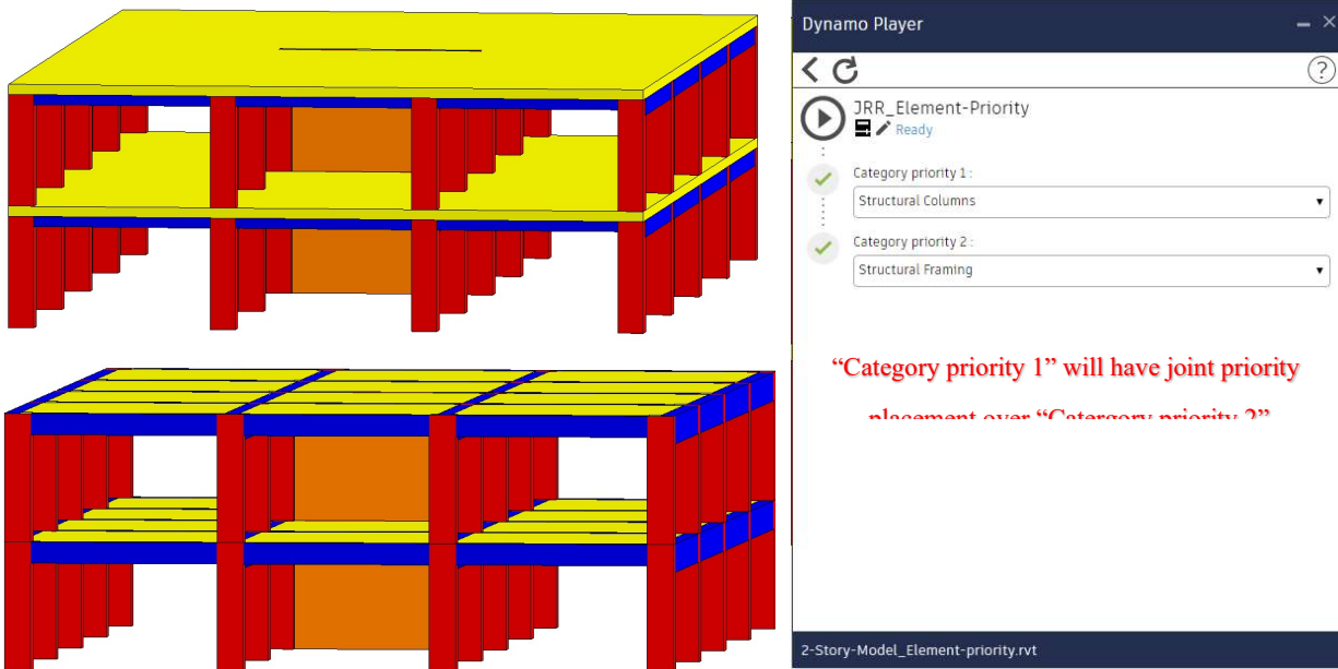
Figure 3.18. Results of running Dynamo script to switch element priorities
