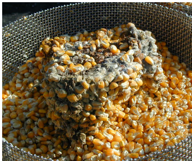
Figure 3. Hot spot formation in one of the layers in the hot spot module.
