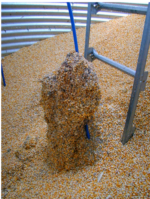
Figure 12. Hot spot detected at the center of the stored grain bulk (temperature cable in the hot spot was previously located 0.3 m away but probed in after the hot spot was detected due to musty smell in the headspace).
