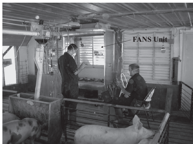
Figure 2. In-field fan calibration with the FANS unit, a portable fan tester.
