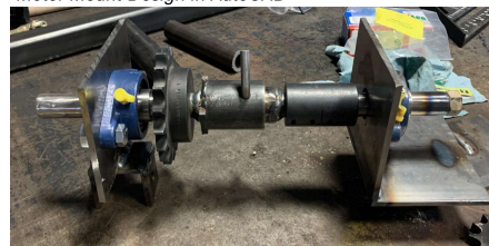
Completed Motor Mount: One side using additional shaft and welded on nut for testing purposes.
