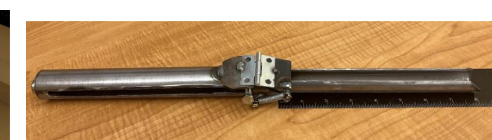
Figure 2 (above): Shielded probe without linear actuator.
