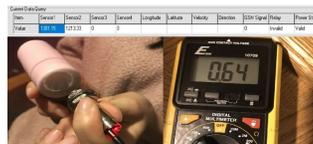
Glued two magnets to small fan to test tachometer. Bit output of 1301 implies VAIN = 0.65V; meter read 0.64V at F/V converter, so values were read correctly. 0.65V → 26 Hz → fan runs at 13 Hz. Seems reasonable but need to validate in future
