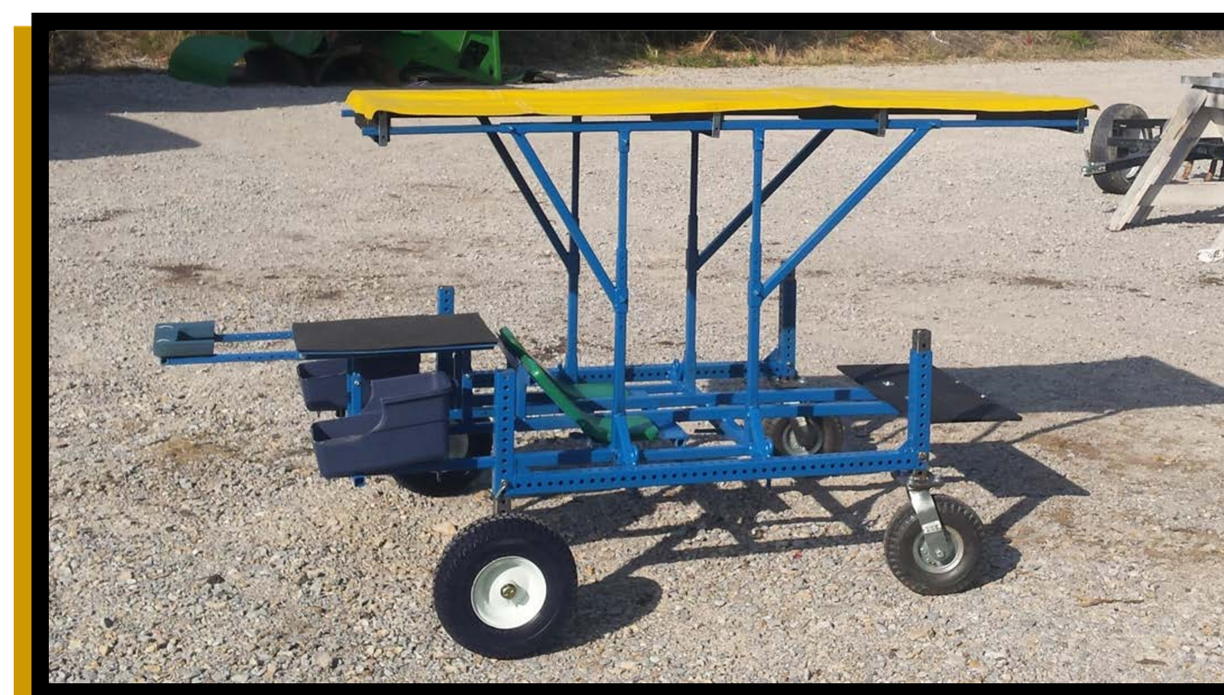
Figure 4: Garlic cart after revisions (low height setting) 6" ground clearance
