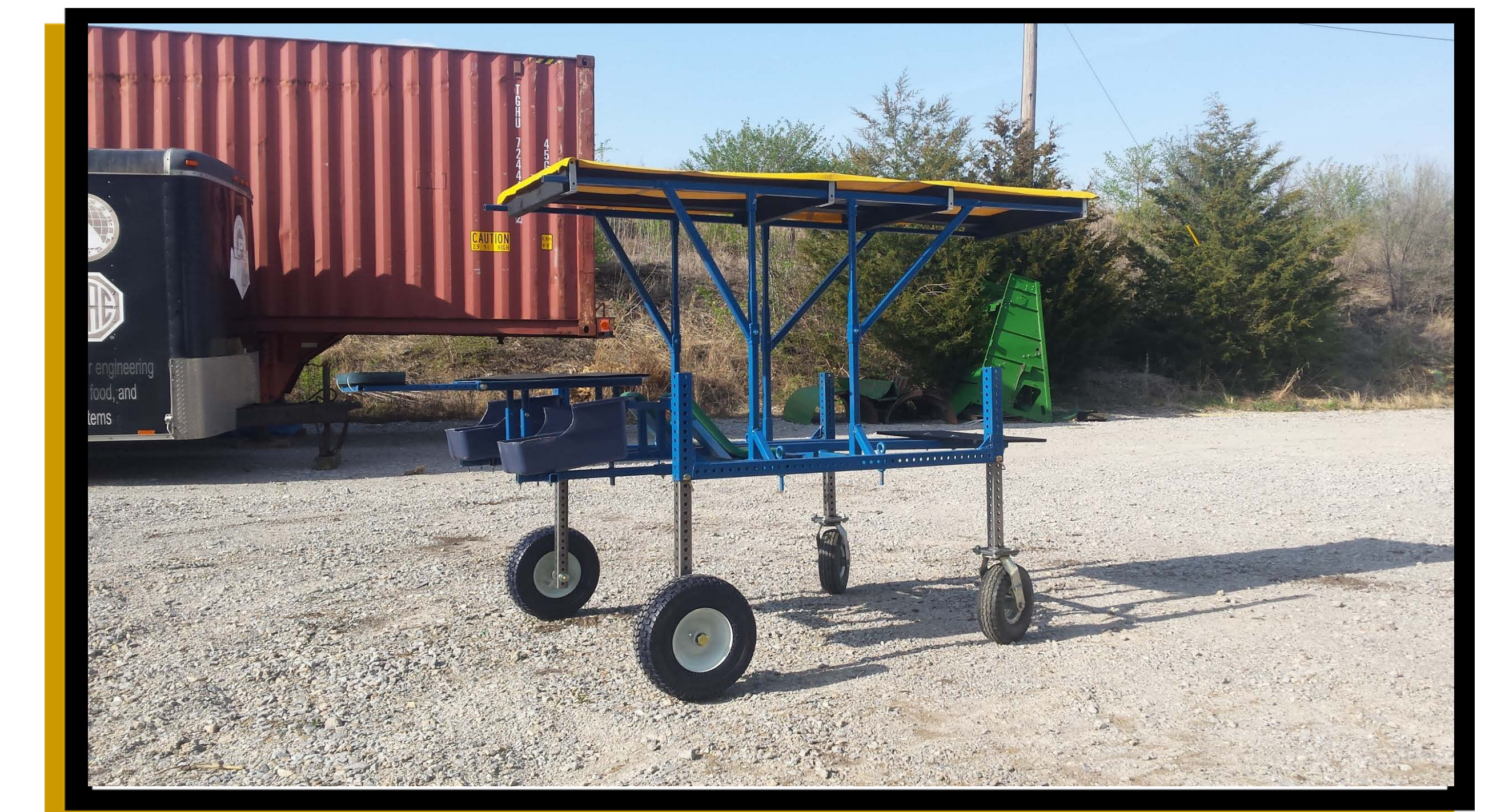
Figure 4: Garlic cart after revisions ( high height setting) 24" ground clearance
