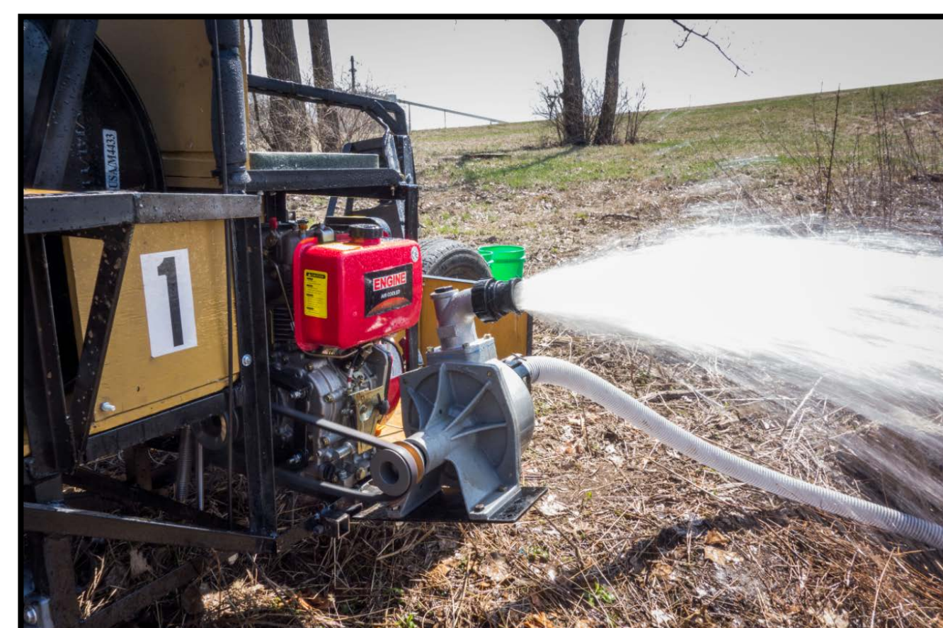
Multiple PTO attachments, including pumping water, provide higher value to stakeholders
