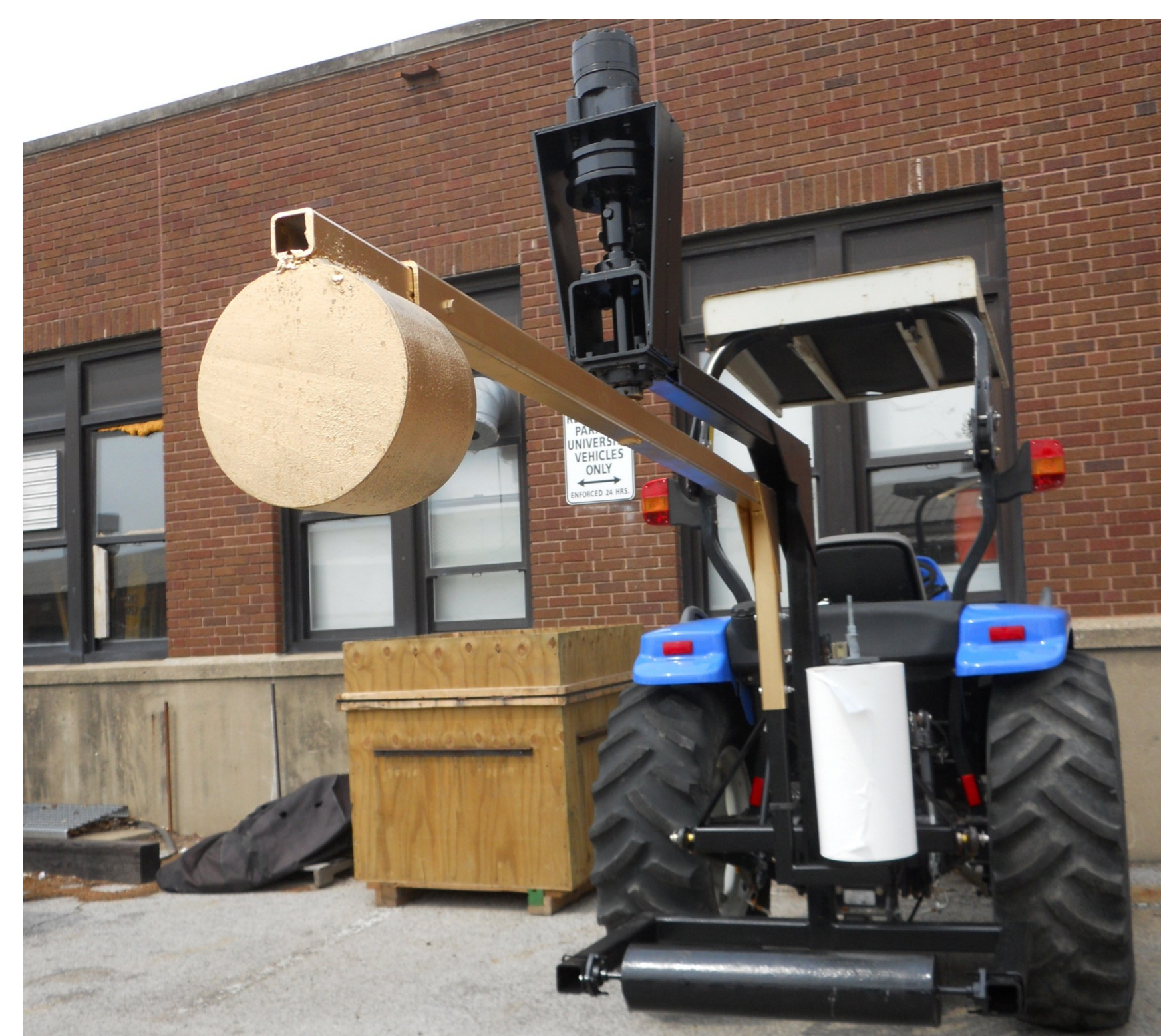
Figure 1. Picture of the nearly completed bale wrapper.
