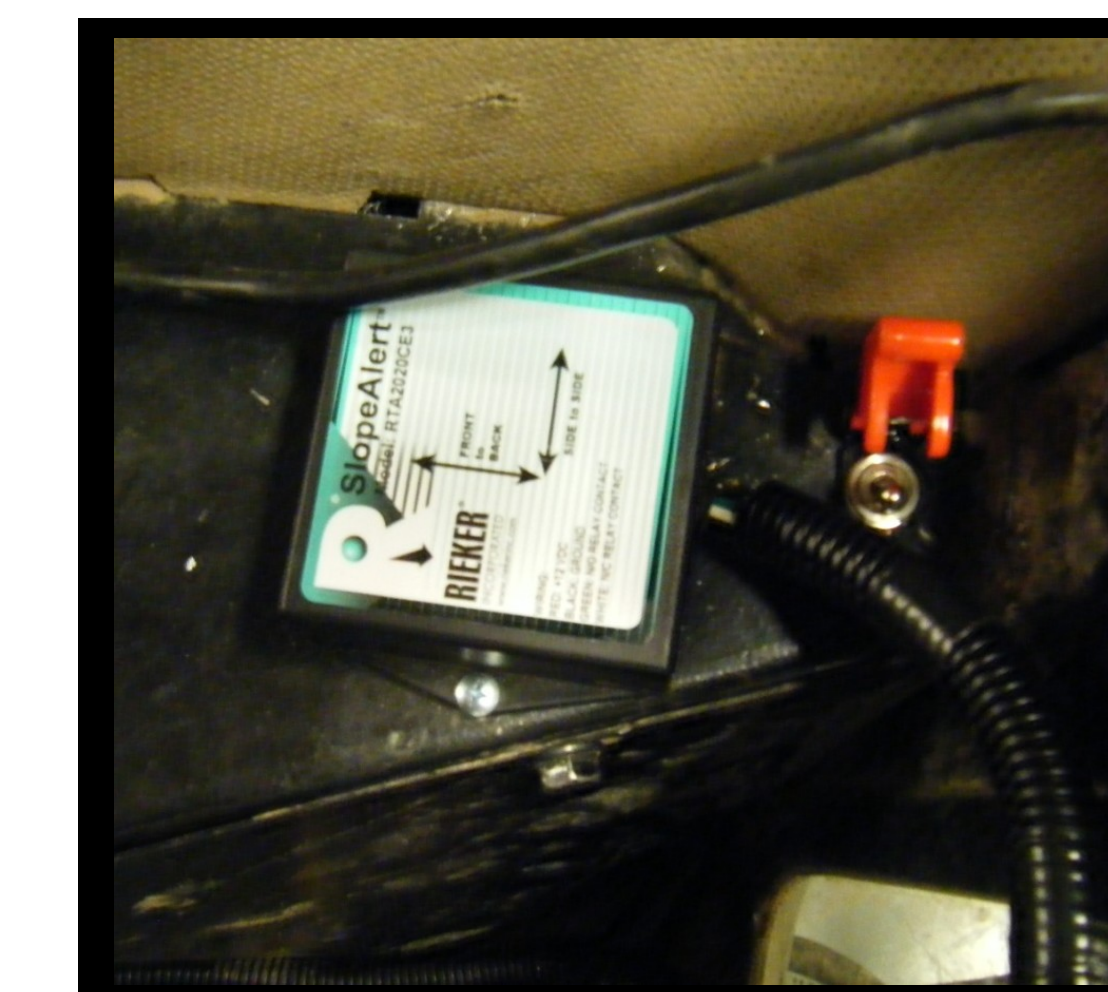
Slope sensor and slope override switch
