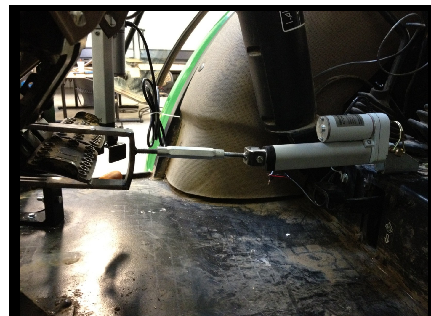
Electric actuator and U-bracket for brakes
