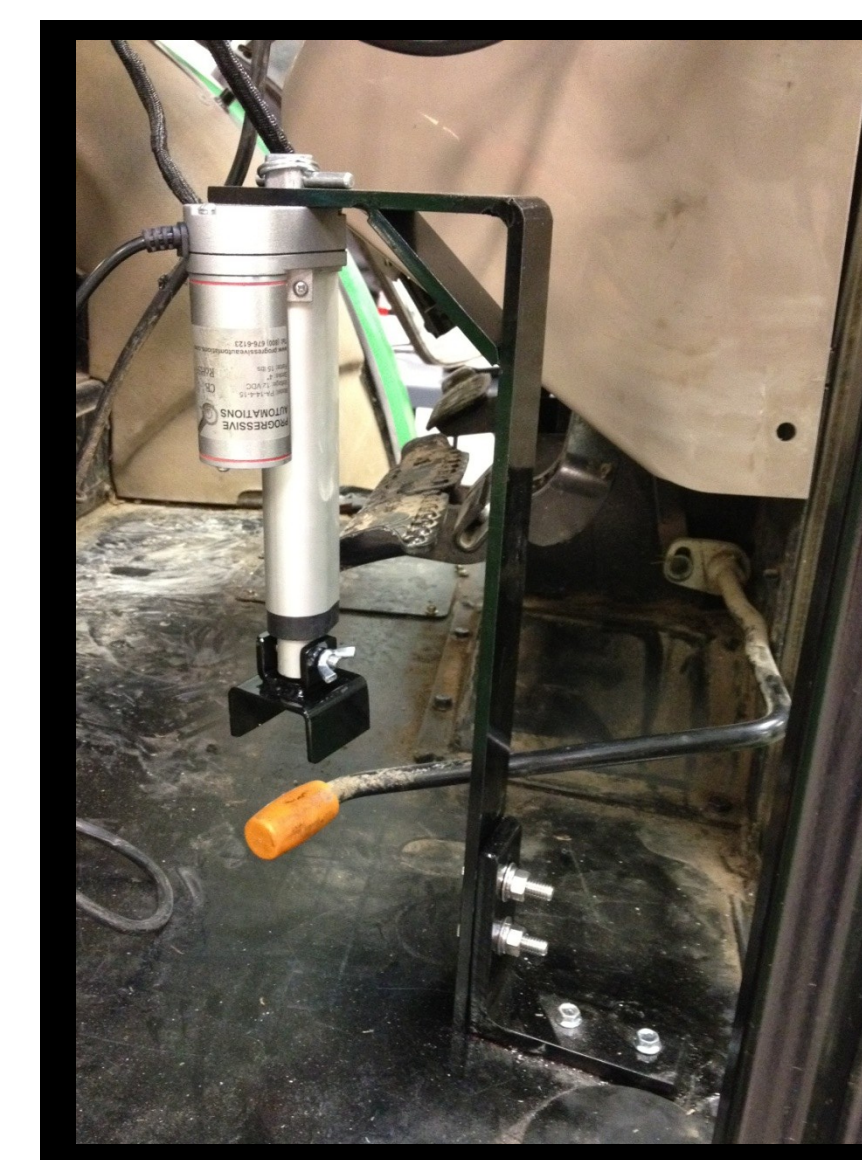
Electric actuator and mounting bracket for throttle
