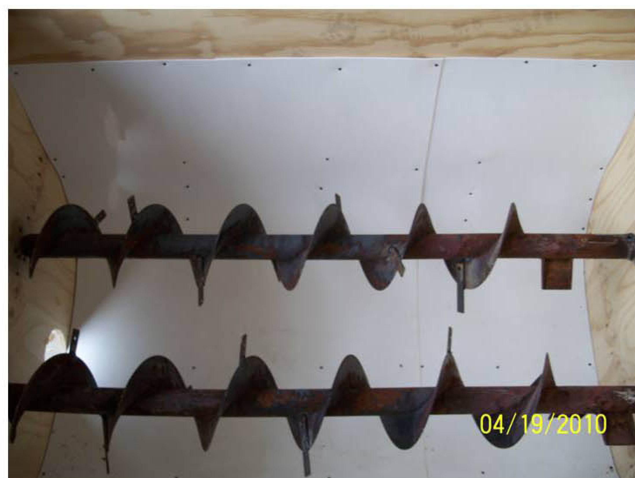
Agitating Auger with Plastic Sheets in place
