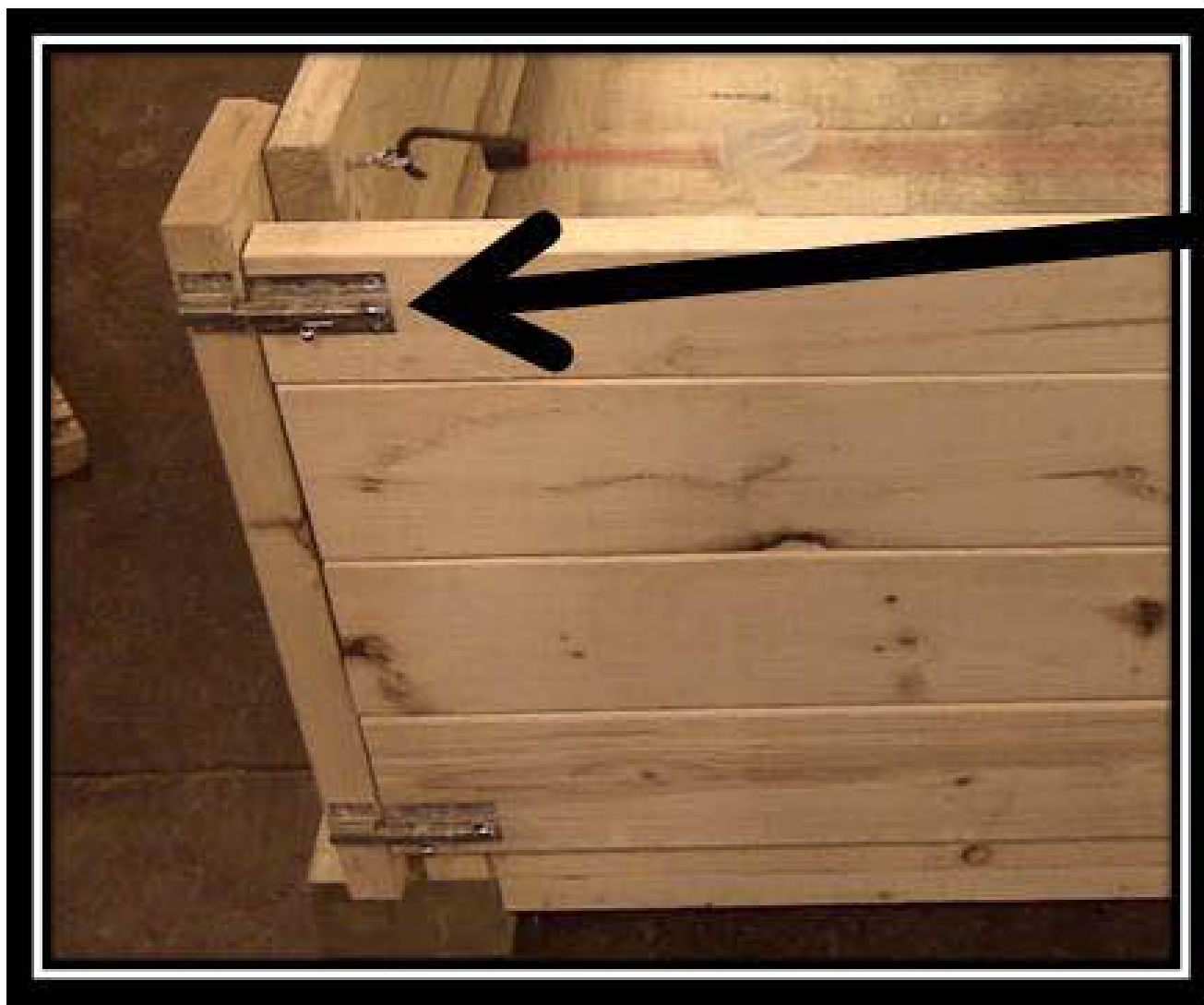
Bolt Locks Used to Hinge Tailgate
