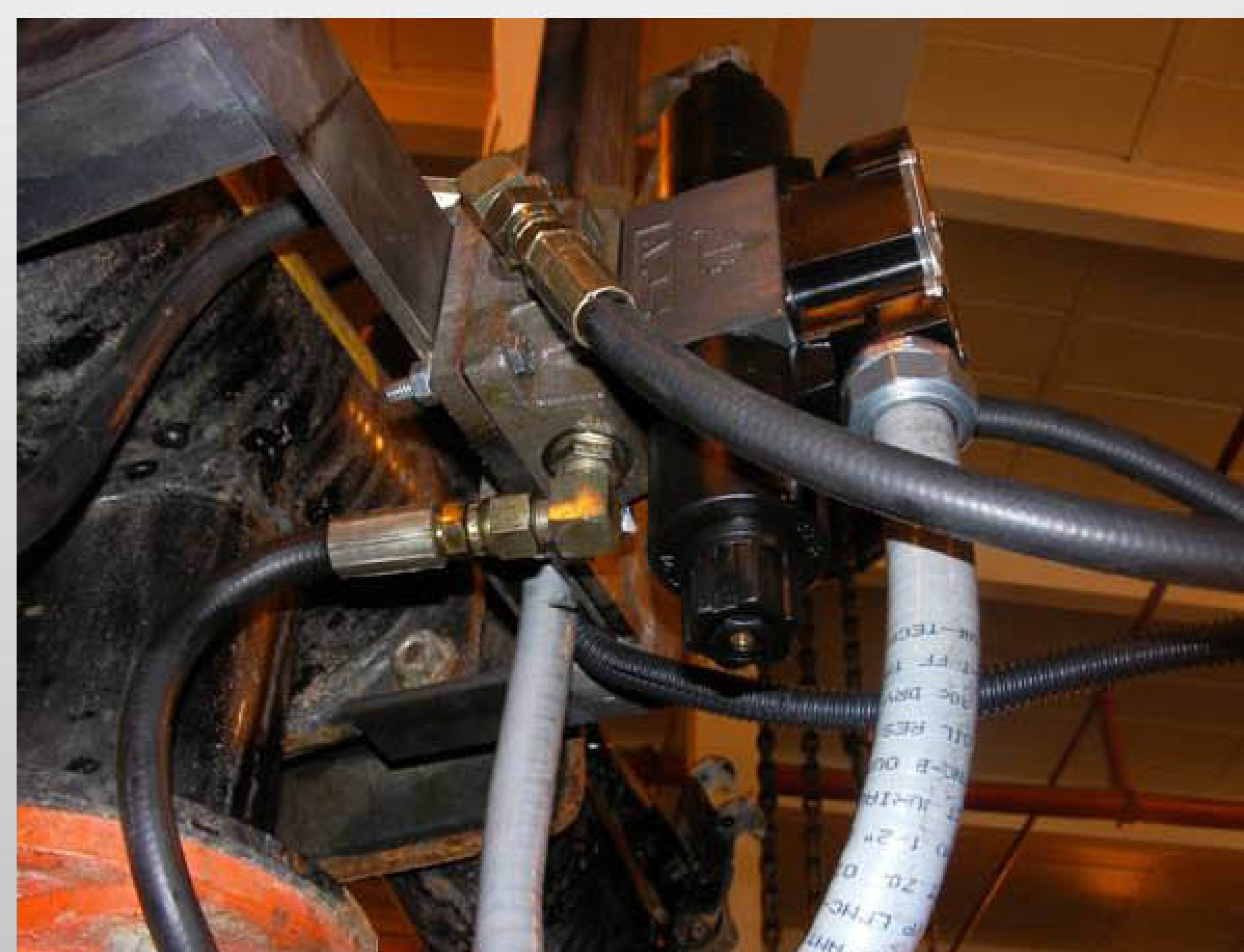
Electro hydraulic valve used to control hydraulic cylinders
