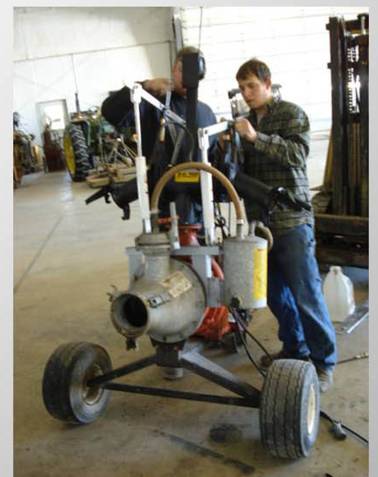
Mounting the cylinders to the manure valves
