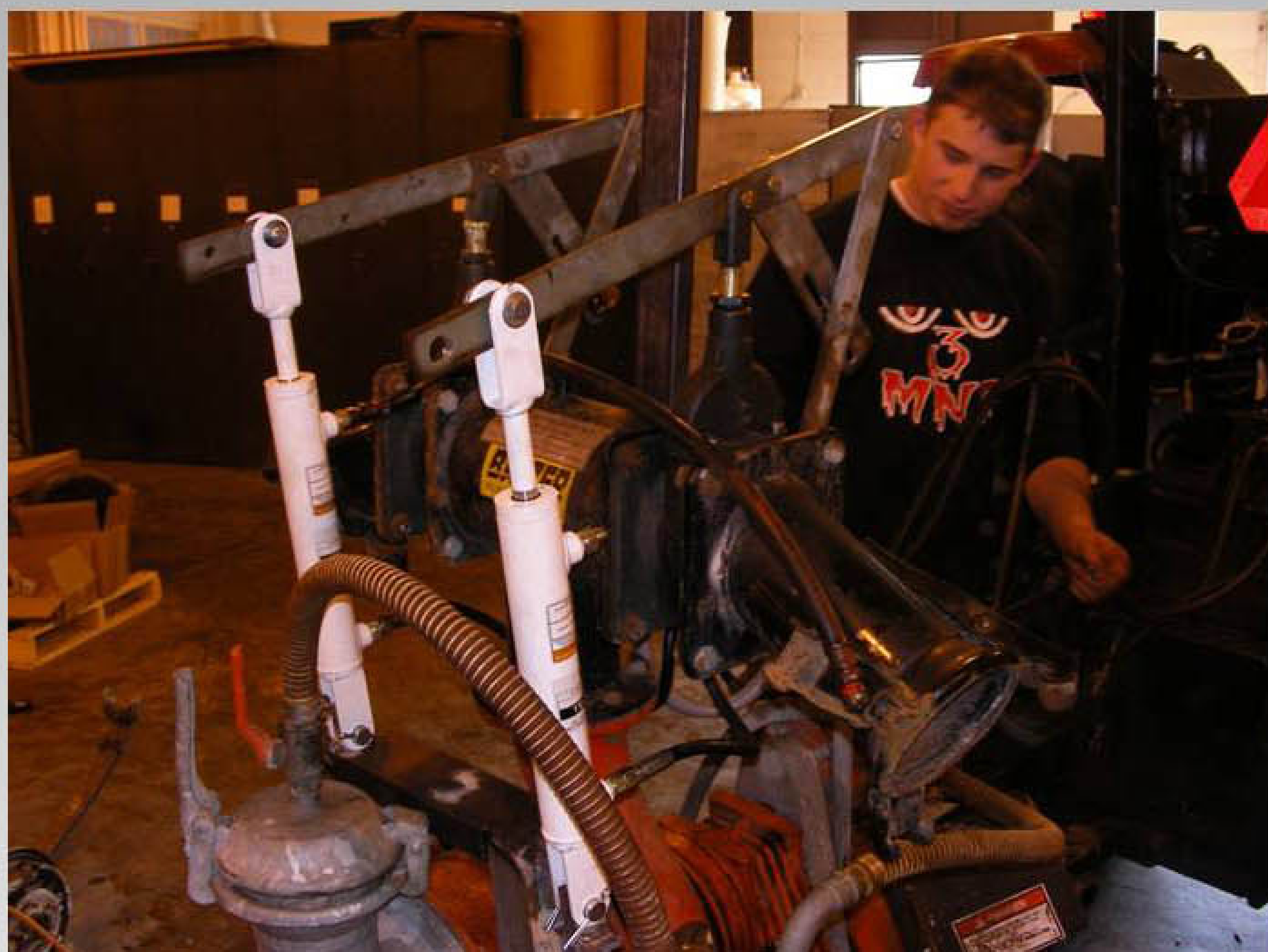
Plumbing the hydraulic cylinders
