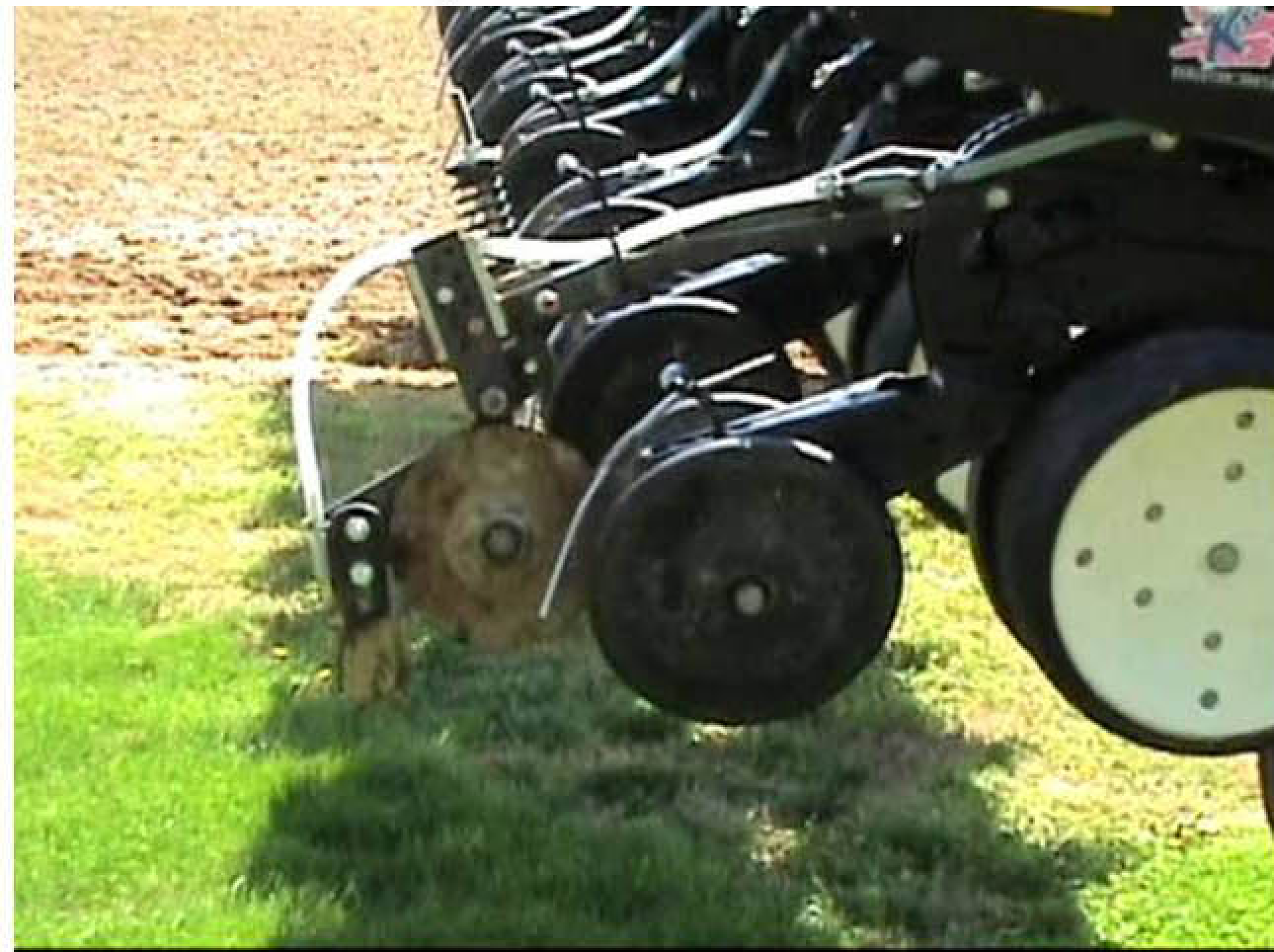
Fertilizer application system mounted to planter unit.
