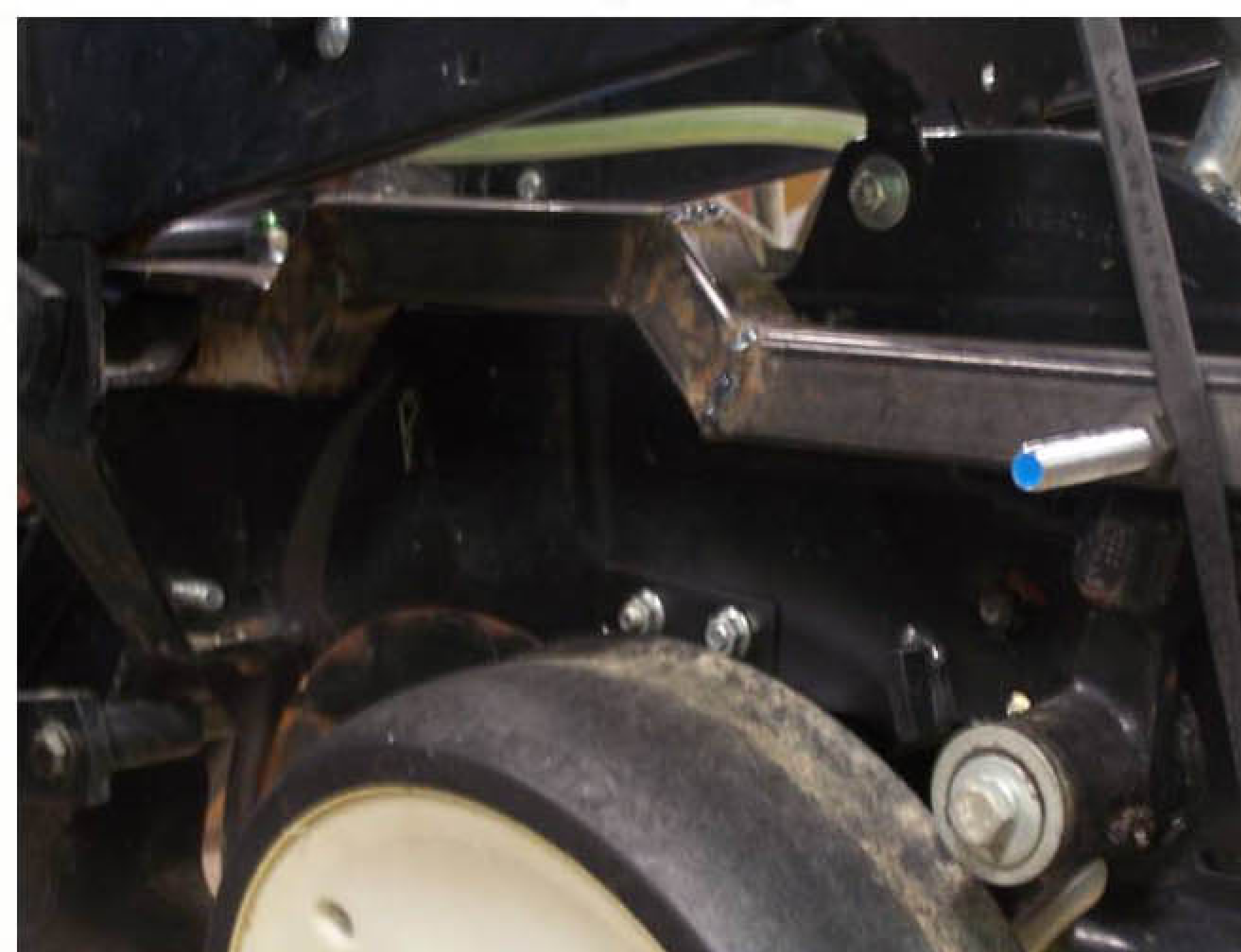
Arched design allowing for full movement of the gauge wheels.
