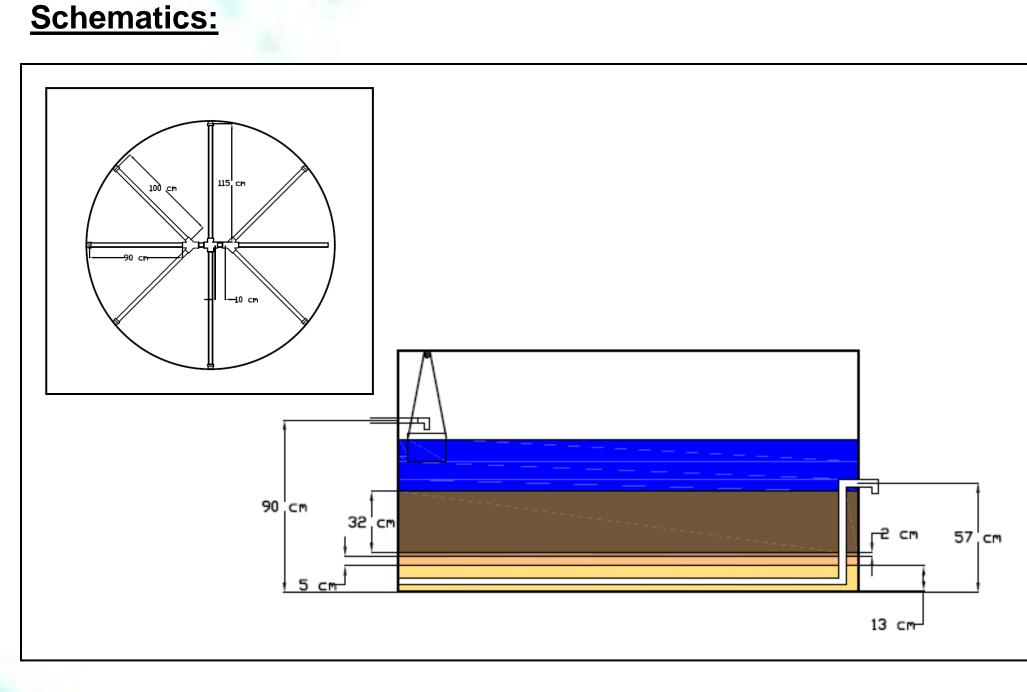
Figure 2: (Left) Schematic of the piped collection system at the bottom of the reactor (Right) cross-section, side view of proposed Bio-Filter Reactor
