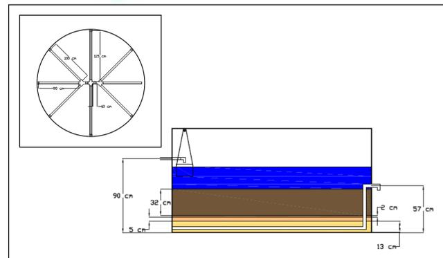
Figure 2: (Left) Schematic of the piped collection system at the bottom of the reactor (Right) cross-section, side view of proposed Bio-Filter Reactor
