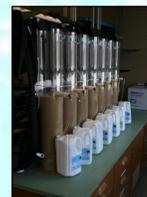
Figure 1: Lab Scale Bio-Filter Reactors
