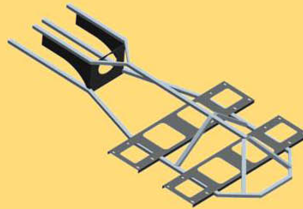
Chrome moly tube frame design
