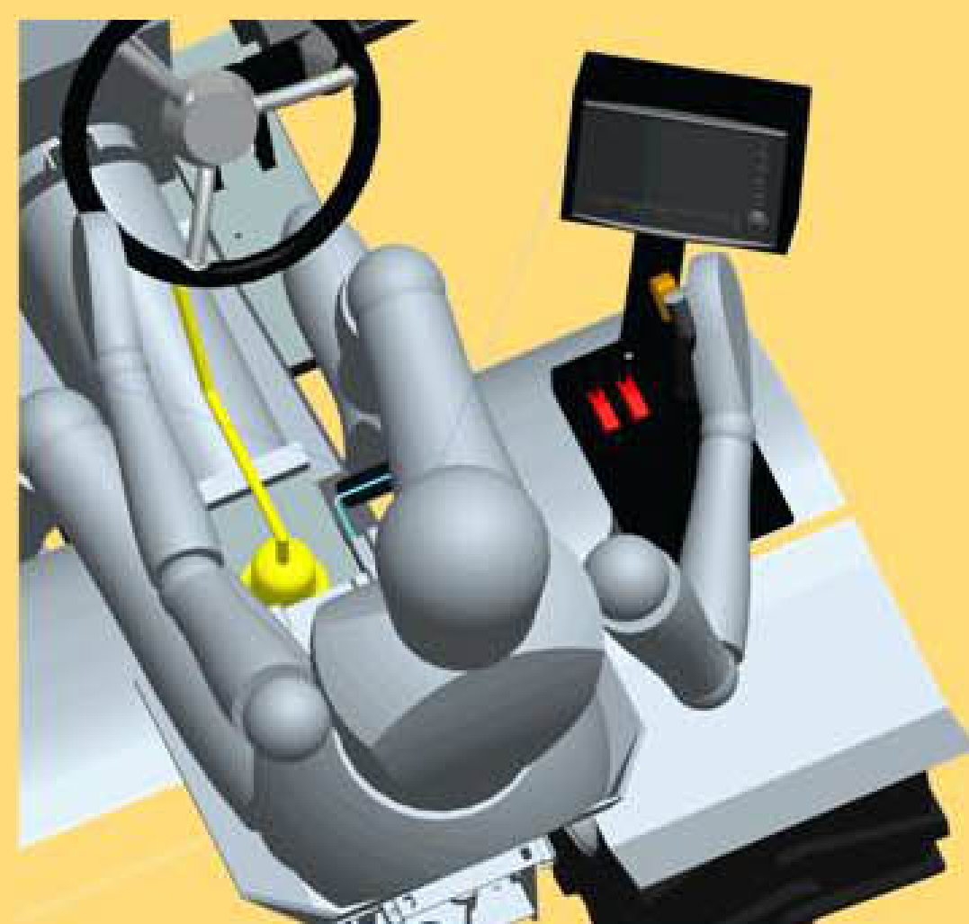
Armrest with finger tip controls and available IQAN mount
