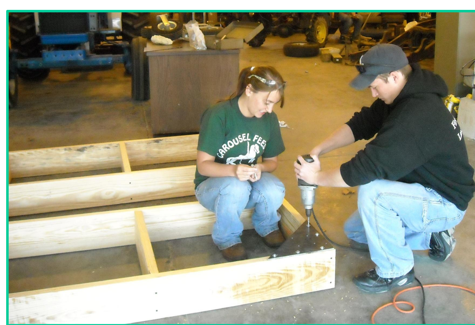
Constructing base frame and attaching mounting plates for casters.
