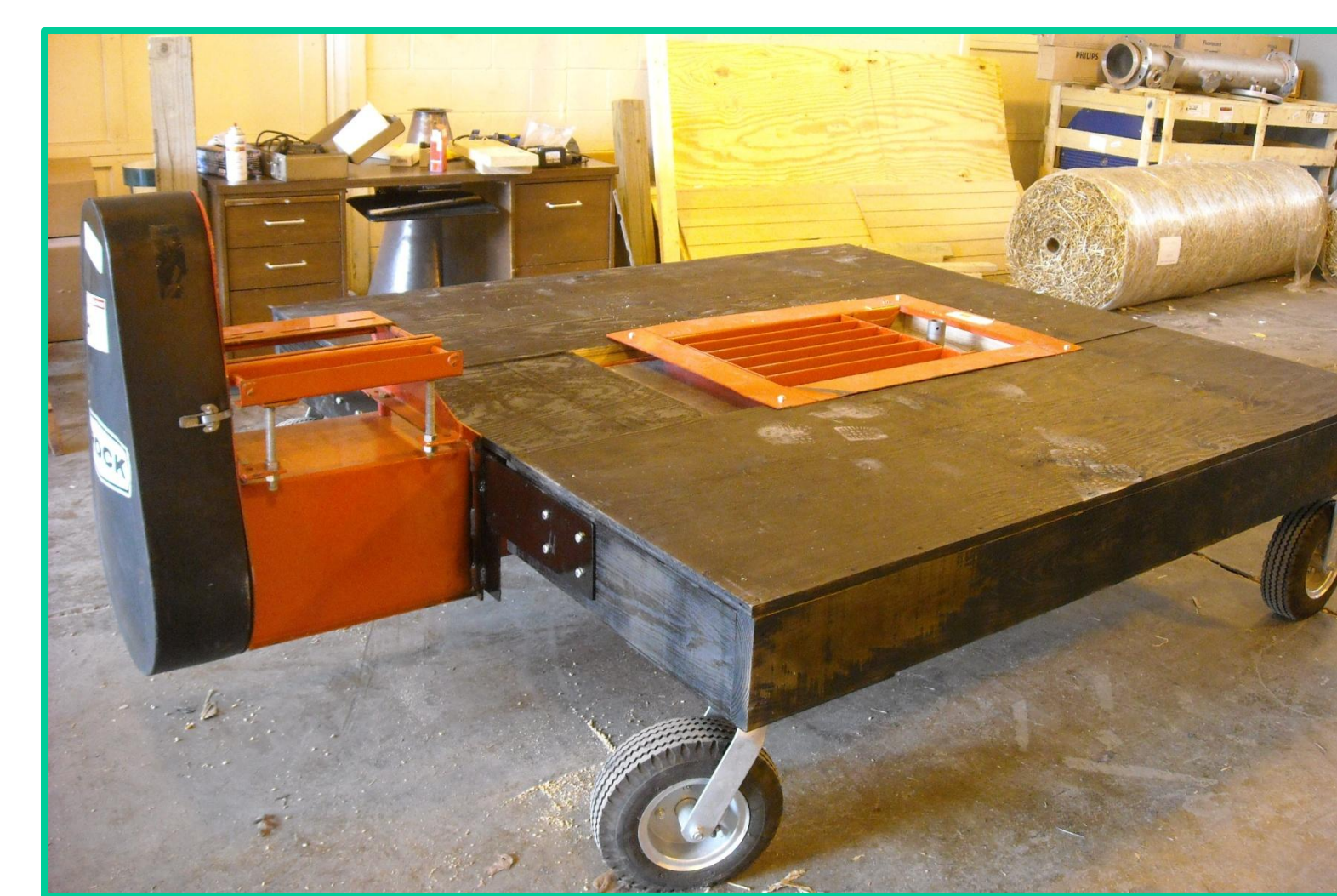
Completed 6.5' x 6.5' base with U-trough auger
