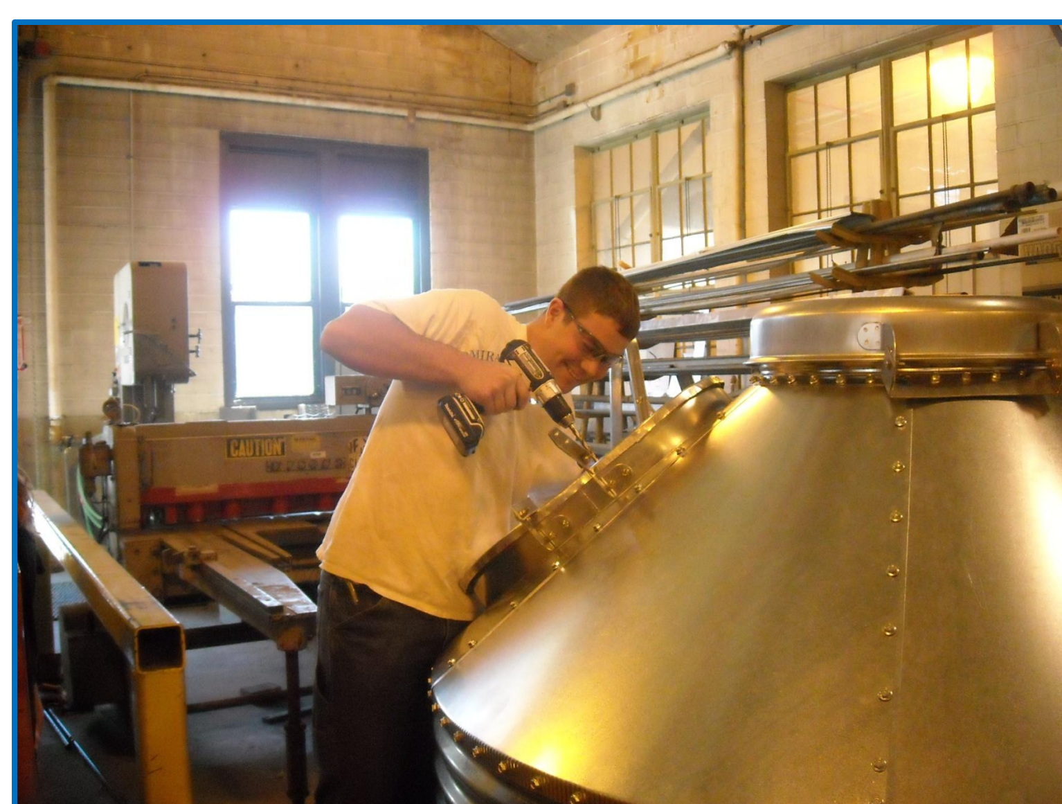
Grain bin assembly and fabrication
