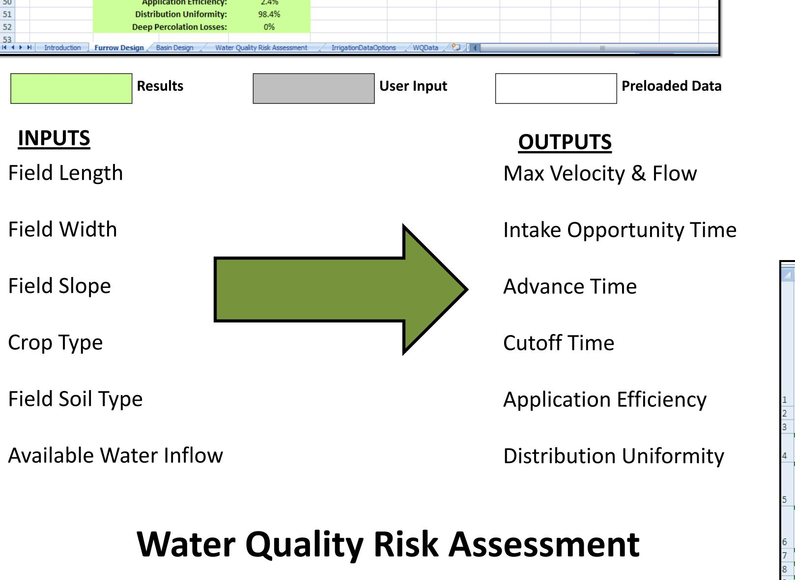
based on the crop being grown. The tool allows them to choose either furrow or basin irrigation, as these are the two most common types of irrigation used in under-developed countries that cannot afford sprinkler or drip systems.
