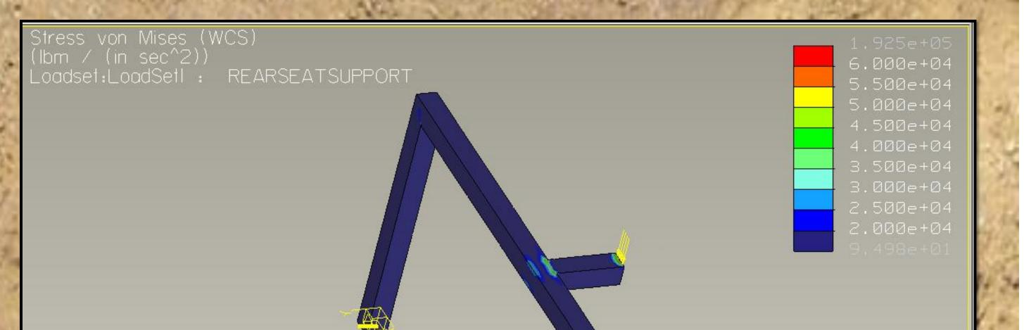
Pro/Engineer and Mechanica were used in the modeling and analysis of the Operator Station. Stress analysis were run on the roll cage and the seat supports. The results of the seat support analysis are shown below. The load was chosen was 750 lbs. This was chosen by taken the weight of the 95 percentile man and multiplying by 3 to simulate a 3g load.
