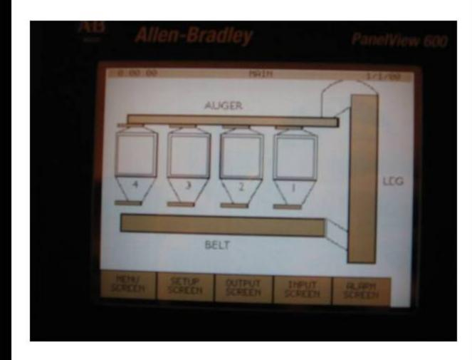
Hazards monitoring systems, provided by 4B Technologies, has been installed throughout the model. Hazards such as; speed monitoring, bearing temperature, grain temperature, belt alignment and bin level are all monitored. This information is transferred to the Watch Dog and T-500 systems. If a hazard is detected, such as a hot bearing, the monitor will send an alarm to the screen and then shut down that specific equipment.
