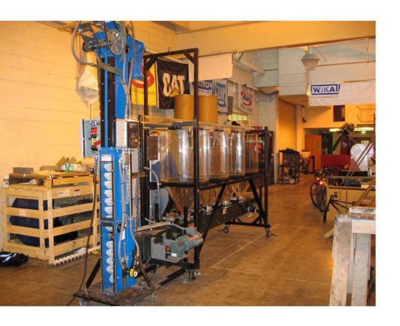
The model contains three different types of conveying systems. The leg is approximately 9 ft tall and was purchased through Universal Conveying Systems. It is rated at 75 Bushels per hour. The belt conveyor was built by Grainway. It is 13 ft long and rated at 100 bushels per hour. The auger was purchased through West Lafayette Agri-Sales in Otterbein, IN. It is rated at 100 bushels per hour.
