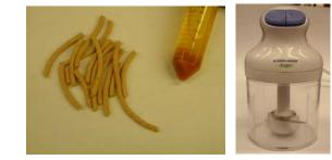
The sample as it comes out of the oil press: extrudate and oil (above left). The small grinder used to break up the extrudate ( above right)
