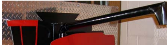
The actuator to the right will retract, extending the unloading auger out as in the picture above.
