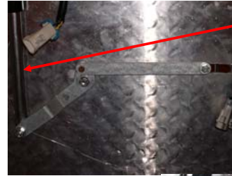
Each set of sieves is controlled by an actuator that is manually adjusted from the cab, and can be preset for certain crops.
