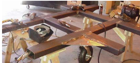
The chassis is supported on four corners by swivel pneumatic castor wheels, and can be fork lifted from all four sides.
