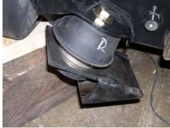
Plans for the actual cab mounting system were used to build mounts that utilized the existing brackets to attach the cab to the chassis.
