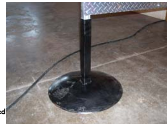
The legs are 20" disk blades welded to steel tubing.
