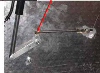
The actuator moves the adjustment arms, causing the sieves to open and close.
