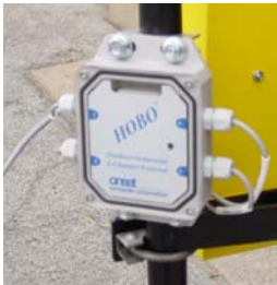
HOBOS data logger. Stores data until data are downloaded onto a PC.
