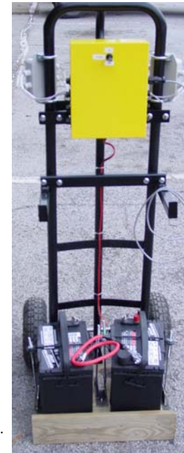
Ground Pressure Sensing Unit Cart. Makes the unit self contained.
