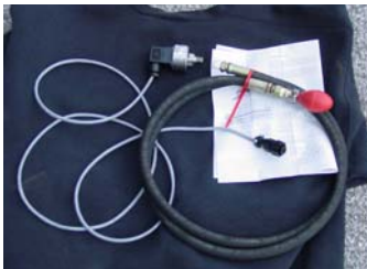
Pressure Sensing Bulb, Hose, and Pressure Transducer
