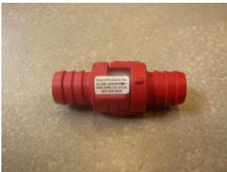
Smart Products, Inc. 300 series check valve, model # 308 1/2 in barbed fitting, both ends Cracking pressure 0.5 PSI
