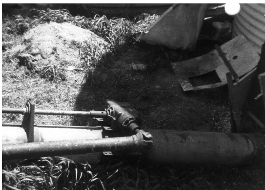
Figure 2. Auger with exposed top shaft and implement input connection (IIC) components.
