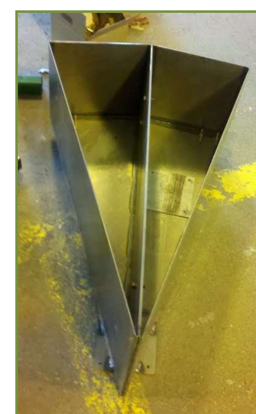
Figure 4: The collection bins, the wide part sits on casters and the point is mounted on a bearing allowing for it to swing into position under the return elevator.
