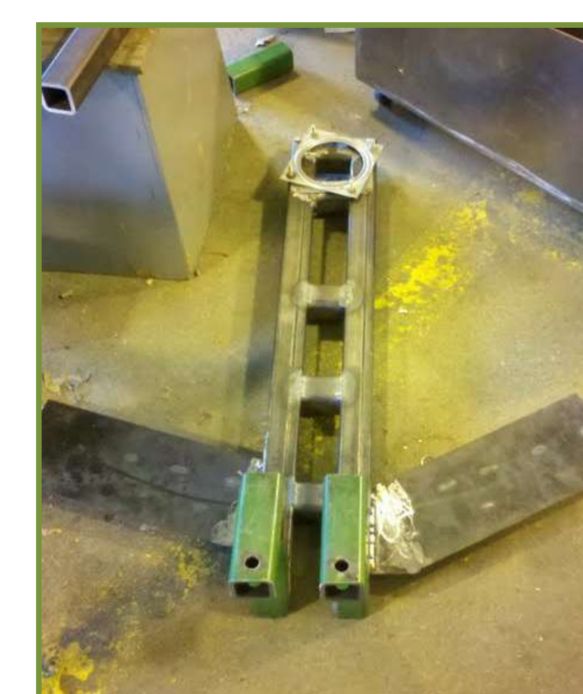
Figure 6: This shows the new clean out door (top), the new slide gate that allows the grain to flow out of the elevator and into the bins, and the support for the slide (bottom).
