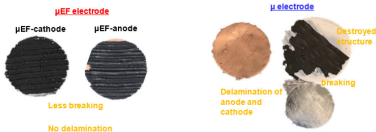
The structured electrode remains intact under mechanical pressure
