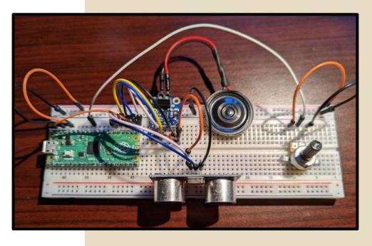
Build a theremin using an ultrasonic sensor
