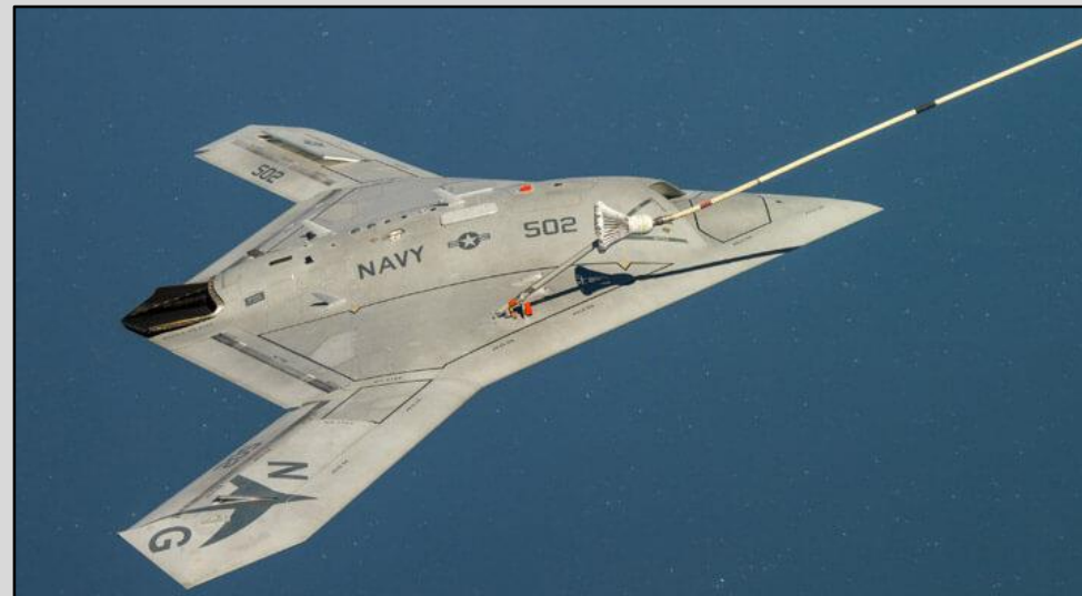
Northrop Grumman X-47B: Autonomous aerial refueling
