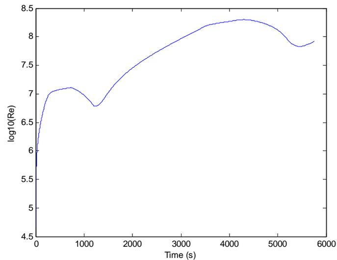
**Fig. A.4.2.1.3.14:** Change in the balloon's East-West horizontal Reynolds number over time.
