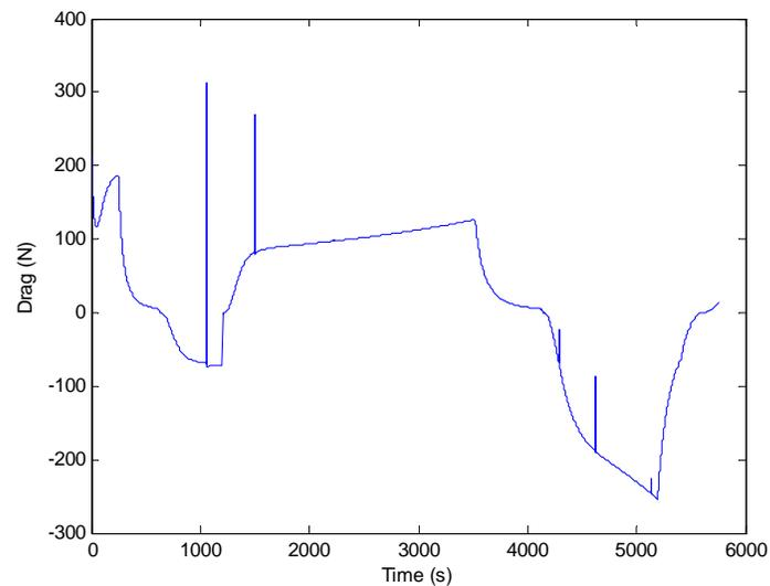
**Fig. A.4.2.1.3.12:** Change in the balloon's East-West drag over time.
