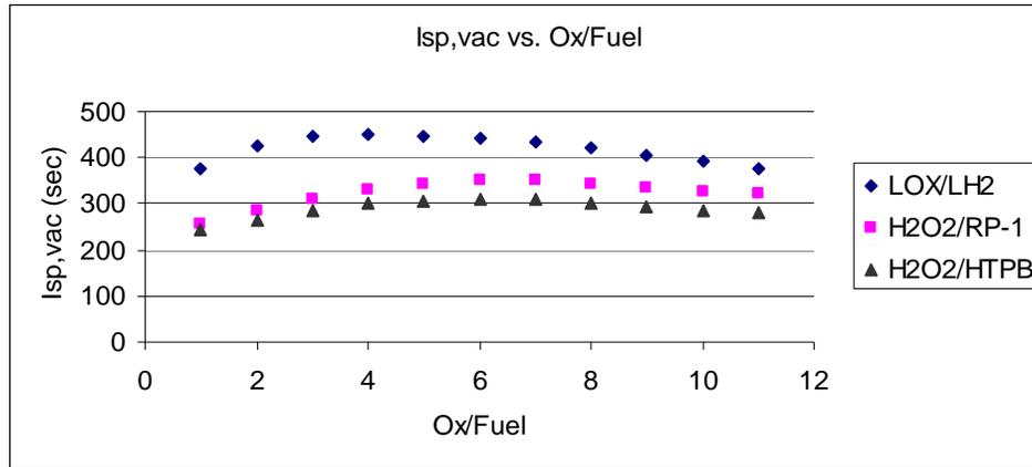
**Fig. Section A.4.2.2.5.2.2:** Vacuum Isp versus oxidizer to fuel ratio.
