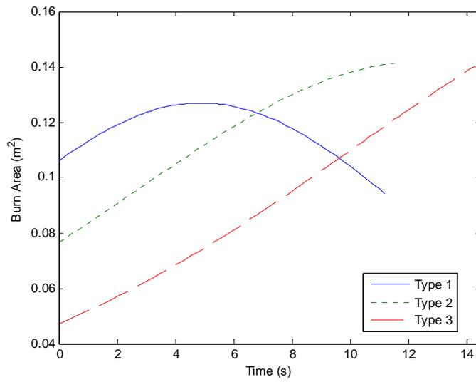
**Figure A.4.2.7.3.4:** Burn area profiles for test geometries.
