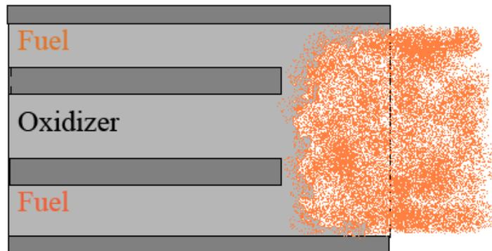
**Figure A.4.2.4.3.1:** Concentric tube injector for liquid fuels.
