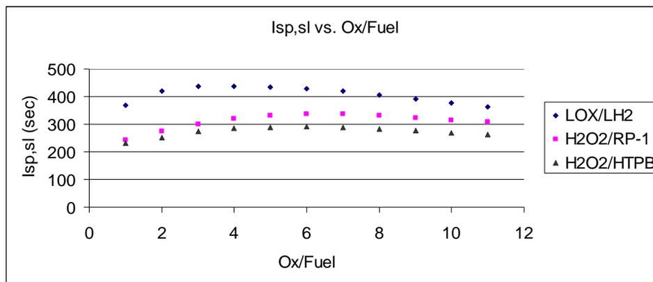
**Fig. Section A.4.2.2.5.2.1:** Sea level Isp versus oxidizer to fuel ratio.
