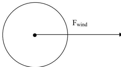
**Fig. A.4.2.1.3.2.4:** Horizontal free body diagram of the balloon
