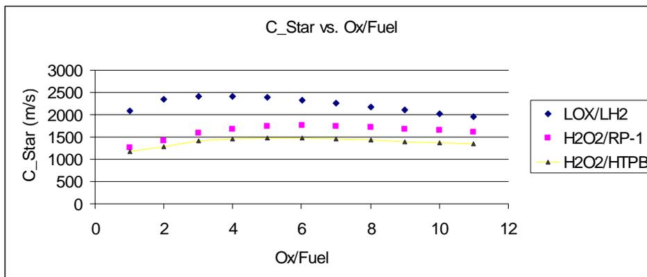
**Fig. Section A.4.2.2.5.2.3:** Characteristic velocity versus oxidizer to fuel ratio.
