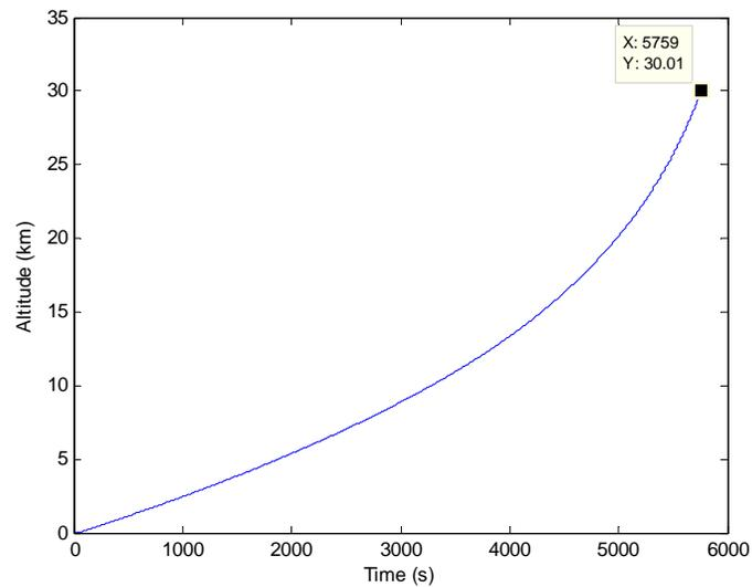
**Fig. A.4.2.1.3.8:** Change in the balloon's altitude over time.
