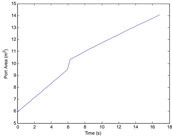
**Figure A.4.2.7.2.5:** Port area profile for test geometry.
