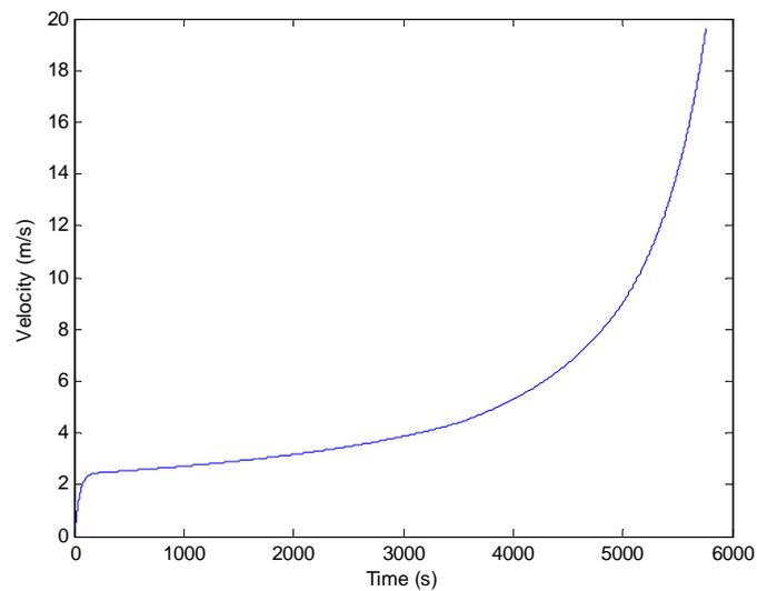
**Fig. A.4.2.1.3.5:** Change in the balloon's vertical velocity over time.
