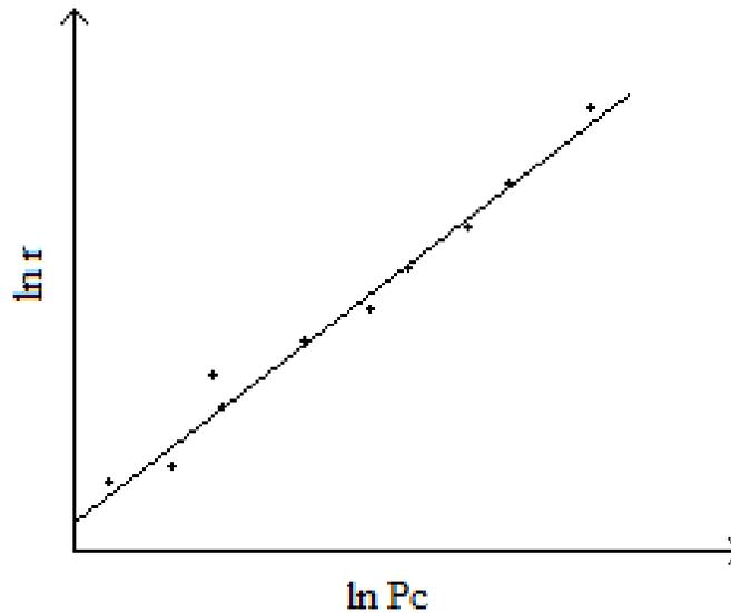
**Fig. A.4.2.7.3.2:** Plot of burning rate test data.
