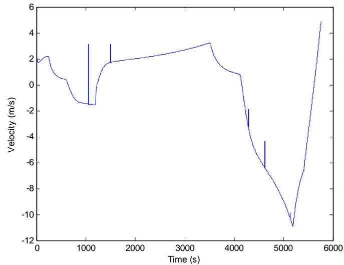
**Fig. A.4.2.1.3.11:** Change in the balloon's East-West velocity over time.
