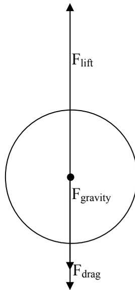
**Fig.A.4.2.1.3.1:** Vertical free body diagram of the balloon.
