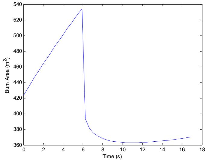
**Figure A.4.2.7.2.4:** Burn area profile for test geometry.
