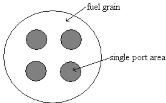
**Fig. A.4.2.7.2.1:** Top-down view of hybrid fuel grain.
