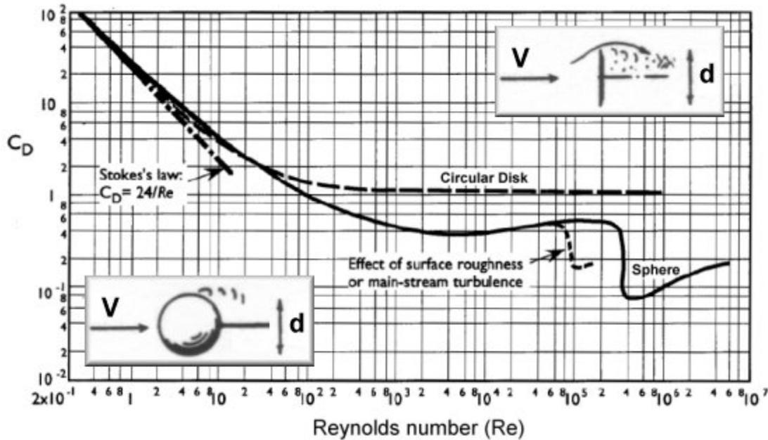
Fig. A.4.2.1.3.15: Drag coefficient of a sphere at varying Reynolds numbers.
