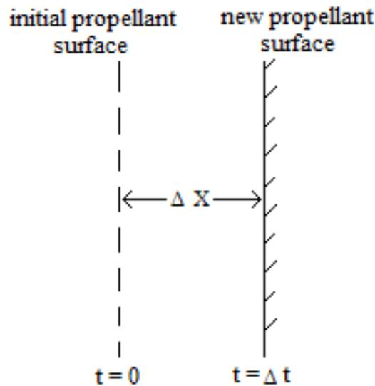
**Fig. A.4.2.7.3.1:** Diagram of burning rate definition.
