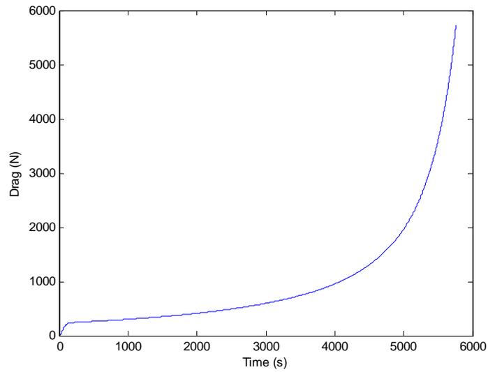
**Fig. A.4.2.1.3.7:** Change in the balloon's vertical drag over time.
