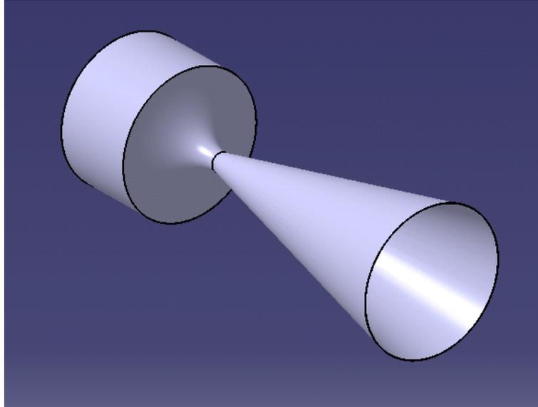
**Figure A.4.2.5.2:** Conical Nozzle CAD
