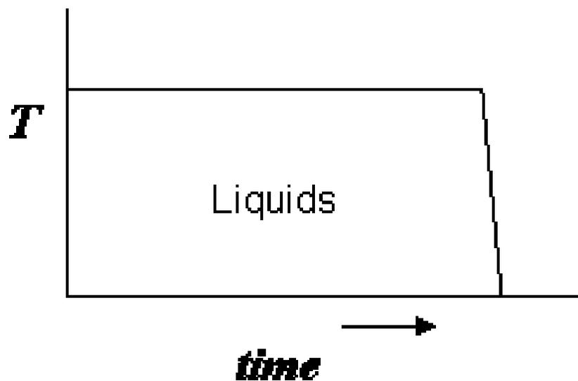
Fig. A.4.2.6.1.1 Thrust-time curve of burned liquid propellant.
