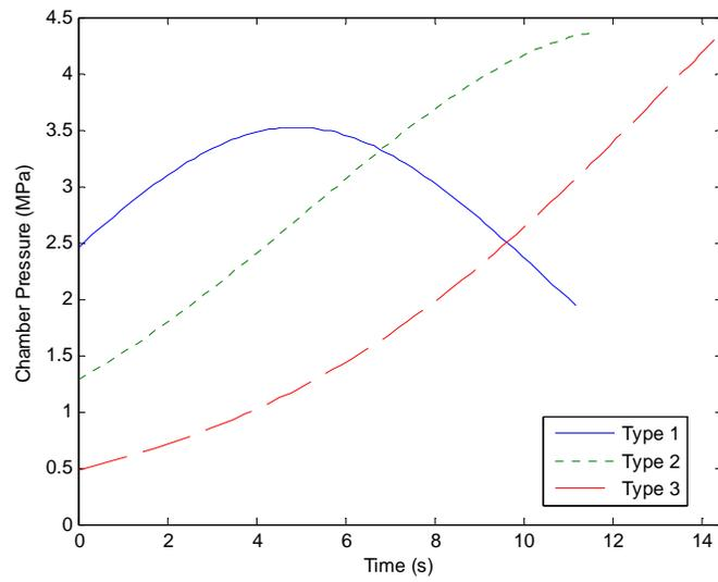
**Figure A.4.2.7.3.5:** Chamber pressure profiles for test geometries.
