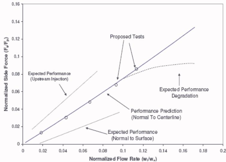
Fig. A.4.6.2.1 Side Force over Primary Force vs. Side Flow Rate over Primary Flow Rate for LITVC<sup>2</sup>
