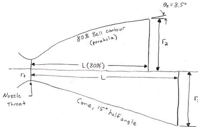
**Figure 4.2.5.1:** Bell Nozzle design based on conical nozzle shape
