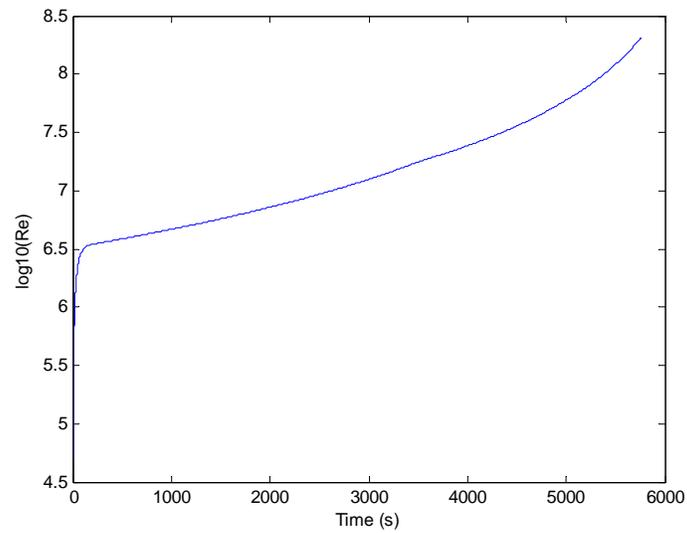
**Fig. A.4.2.1.3.13:** Change in the balloon's vertical Reynolds number over time.
