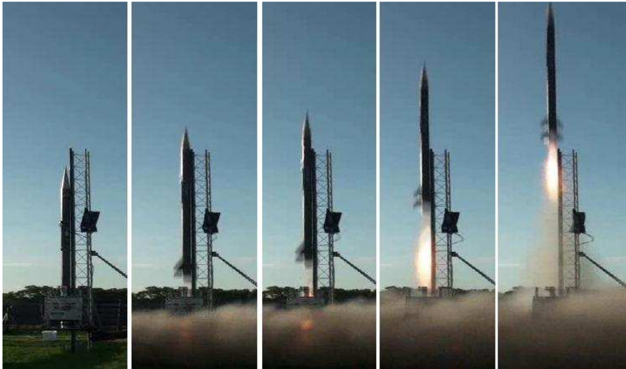
Figure 24. Snapshots of hybrid flight-vehicle clearing launch tower under 6 Gs of acceleration, in ~0.4 sec.
