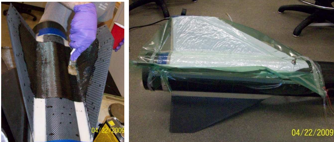
Figure 13. Carbon-fiber wet hand layup (left) and vacuum bagging of fin assembly (right)
