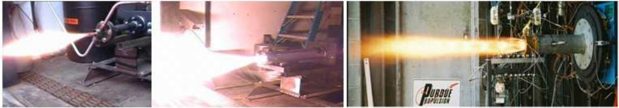
Figure 2. Heritage motors for the flight-weight design. Hot-fire tests from the 25 lbf-thrust, 250 lbf-thrust, and 900 lbf-thrust hybrid rocket motors are shown from left to right.
