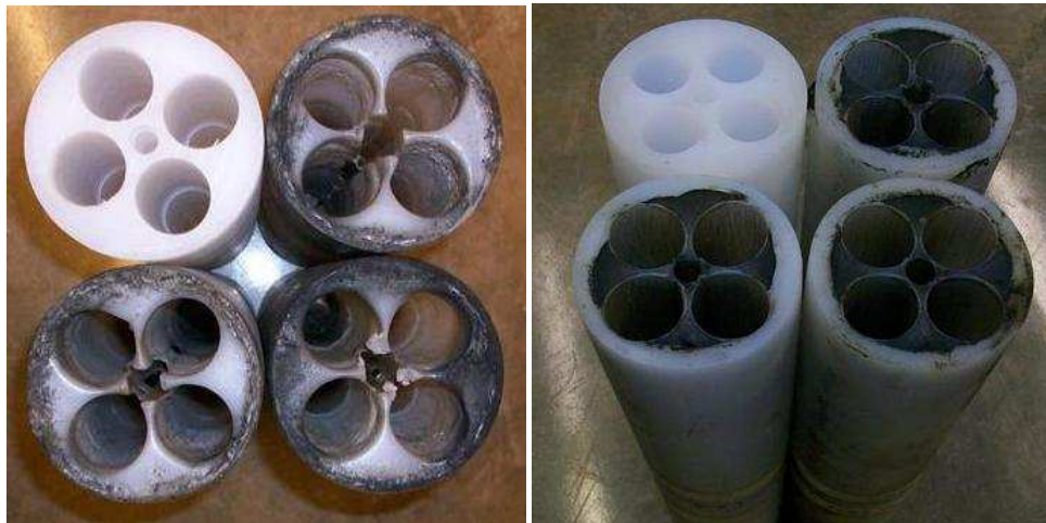
Figure 10: Fuel grains from Hot-fires #4, #5, and the integrated vehicle test along with a new grain. Top view of fuel ports (left image) and bottom view of fuel ports (right image).
