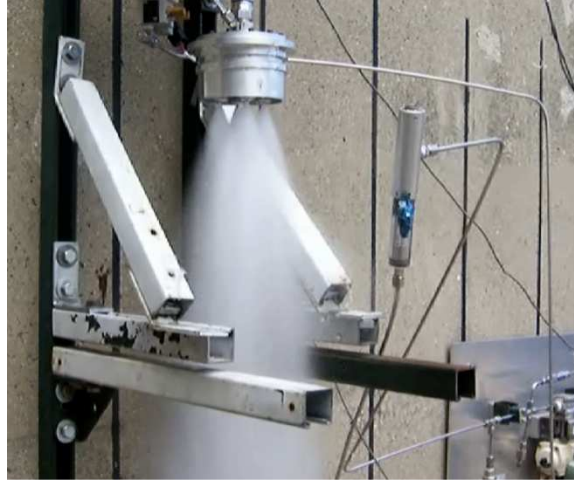
Figure 5. Injector cold flow tests on the flight-weight injector manifold assembly. Notice the disengaged quick-disconnect assembly on the right-hand side of the picture.
