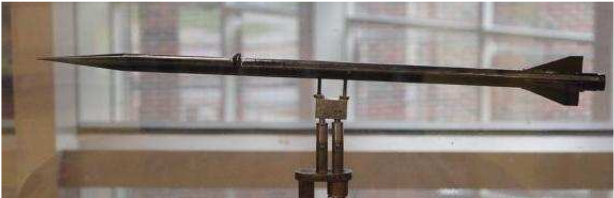
Figure 15. Subsonic wind tunnel testing of sub-scale vehicle model.
