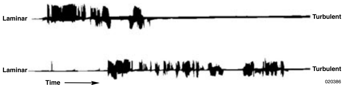
Figure 4.2.3-5. Boundary layer transition from laminar to turbulent for crossflow instability as given by ac-coupled surface hot-film sensor anemometer signals.
