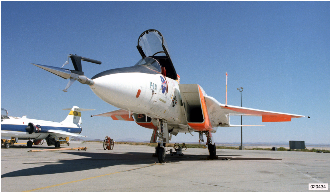
Figure 4.2.5-4. Transition cone mounted in front of test bed aircraft.
