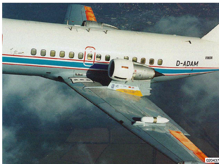
Figure 4.2.2-2. VFW614/ATTAS in flight with NLF nacelle installed on the port engine.
