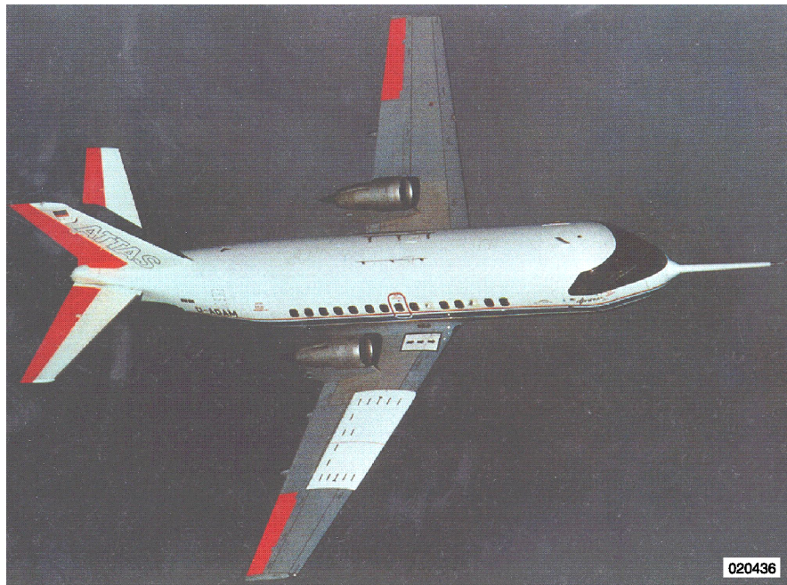
Figure 4.2.1-6. DLR test aircraft VFW614/ATTAS with a glove for natural laminar flow (NLF).
