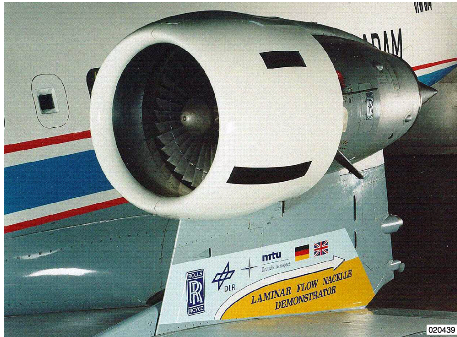
Figure 4.2.2-3. Closeup view of the NLF nacelle on VFW614/ATTAS aircraft.
