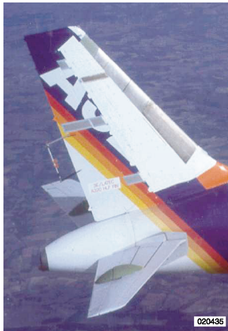
Figure 4.1-3. Vertically movable wake rake at the rudder of the A320 fin.
