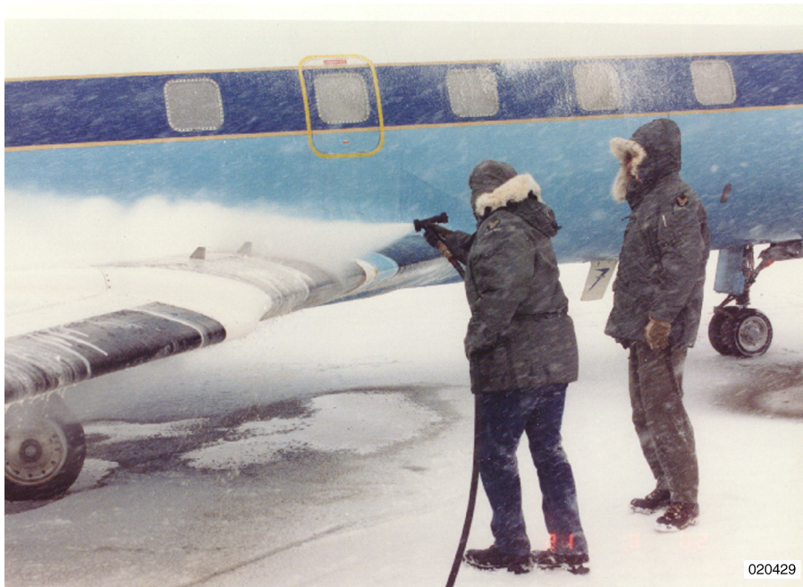
Figure 5.1.2-4. Photo of deicing JetStar LEFT aircraft after overnight freezing rain storm.
