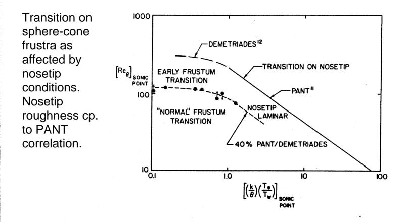
FIGURE 10 Nosetip instability effects on cone frustum transition.
