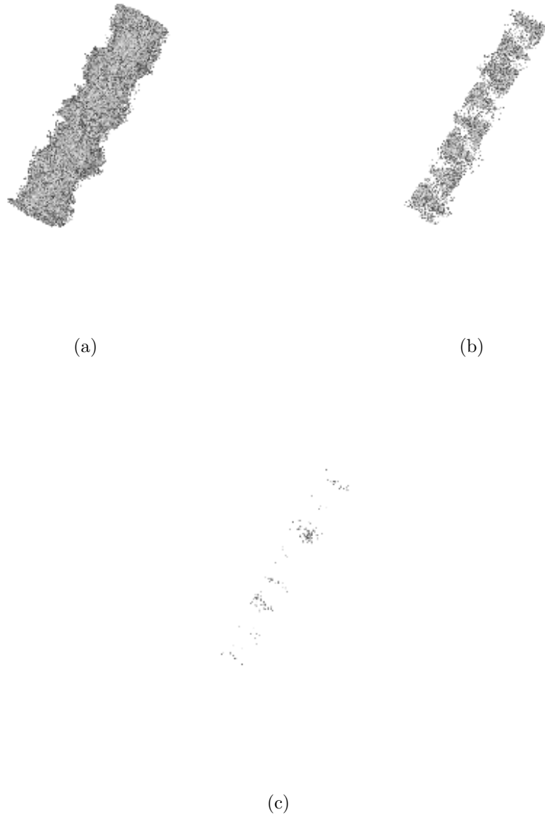
Figure 3.19 Vorticity magnitude isosurfaces for STRN4 at t/T = 45.12 ; (a), (b), and (c) correspond to 0.1, 0.25, and 0.5 times the peak vorticity magnitude respectively
