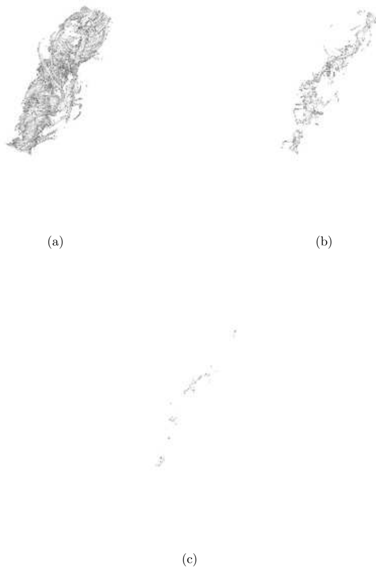
Figure 3.125 Vorticity magnitude isosurfaces for STRN2 at t/T = 103.05 ; (a), (b) and (c) correspond to 0.1, 0.25 and 0.5 times the peak vorticity magnitude respectively
