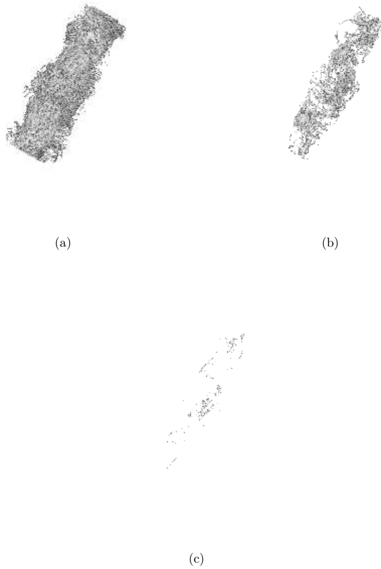
Figure 3.31 Vorticity magnitude isosurfaces for STRN4 at t/T = 100.78 ; (a), (b), and (c) correspond to 0.1, 0.25, and 0.5 times the peak vorticity magnitude respectively
