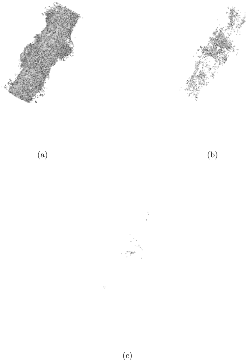
Figure 3.33 Vorticity magnitude isosurfaces for STRN4 at t/T = 104.37 ; (a), (b), and (c) correspond to 0.1, 0.25, and 0.5 times the peak vorticity magnitude respectively
