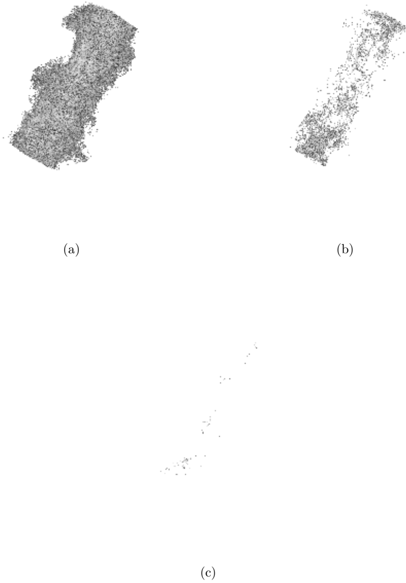
Figure 3.35 Vorticity magnitude isosurfaces for STRN4 at t/T = 107.57 ; (a), (b), and (c) correspond to 0.1, 0.25, and 0.5 times the peak vorticity magnitude respectively
