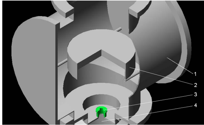
FIGURE 1: Schematics of the experimental set: 1) body of the expansion camera; 2) substrate; 3) nozzle; 4) reactor.
