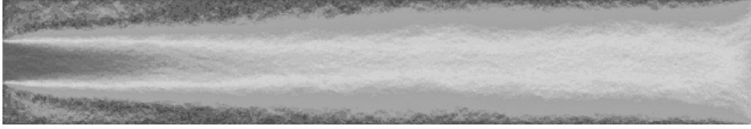
Figure 4. General nature of flow field. Mach contours, time = 4.03 secs.
