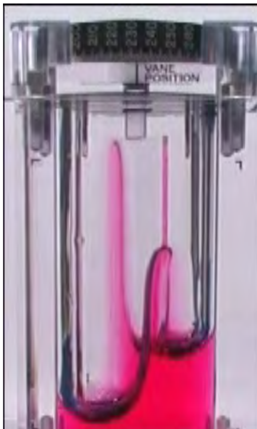
Frame from a video of the “Vane Gap” experiment operating in ISS. Designed by Collicott using the Surface Evolver code.
