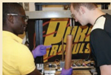
AAE's graduate student Oluwatobi Busari (left) and senior Nicholas Eisenhauer (right) prepare the hybrid grain for the 3D paraffin printer as part of AAE 535. Other students involved in the project are: Alix Crandell, Michael Creech, Michael King, Austin Link, Sarah Marx, and Chris Zaseck. Jason Gabl, Research Engineer in AAE, also helped with the printer development.
