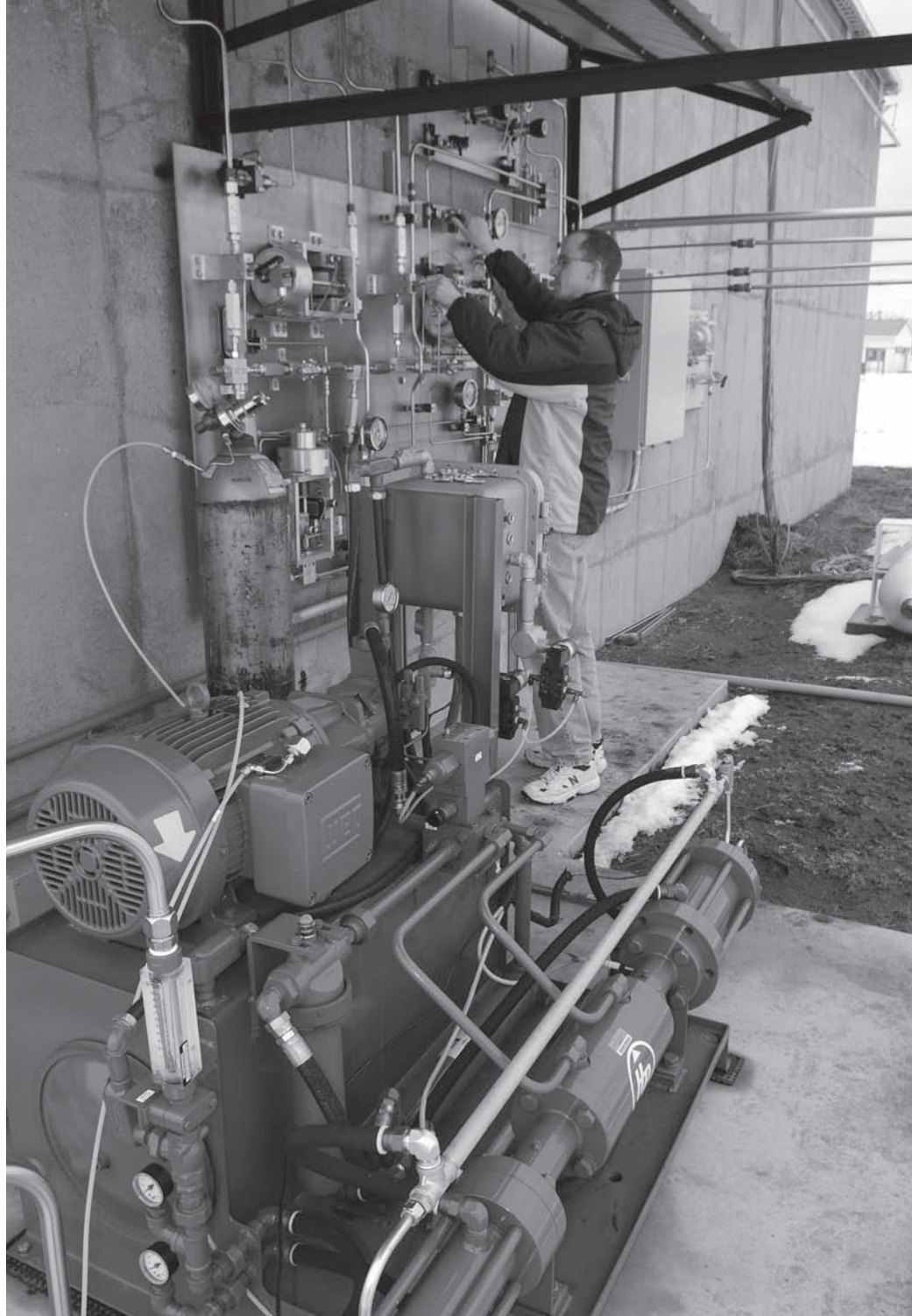
Timothée Pourpoint, a senior research scientist in Purdue's School of Aeronautics and Astronautics, adjusts valves needed to direct the flow of hydrogen and nitrogen in bulk high-pressure hydrogen storage and feed system. (Purdue News Service photo/David Umberger)
